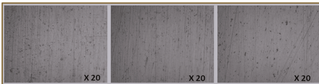
Figure 9. Micrographs of the friction stir layer cut once at a depth of 25 µm at an 800 rpm rotational speed and an 80 mm/min linear speed.
