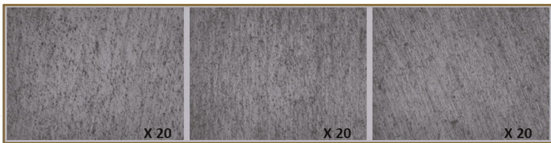
Figure 13. Micrographs of the friction stir layer taken at a single 200 \mu\text{m} cutting depth, 800 rpm rotating speed, and 80 mm/min linear speed.
