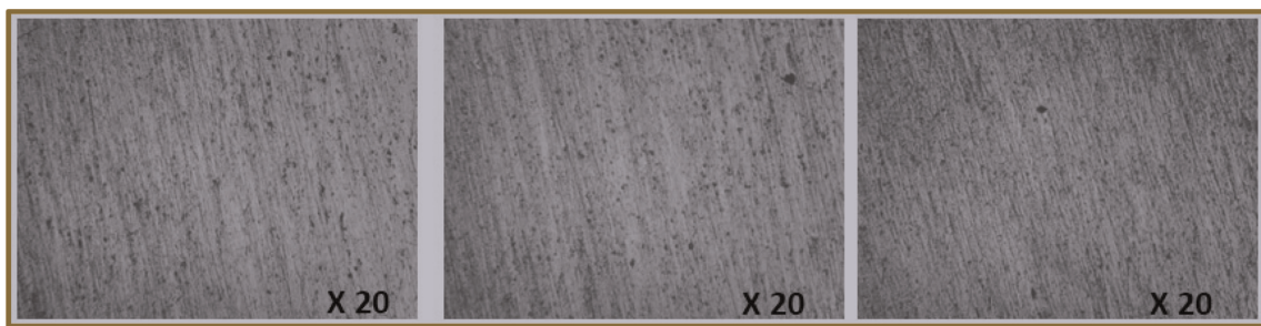
Figure 14. Micrographs of the friction stir layer taken at a single 400 \mu\text{m} cutting depth, 800 rpm rotating speed, and 80 mm/min linear speed.
