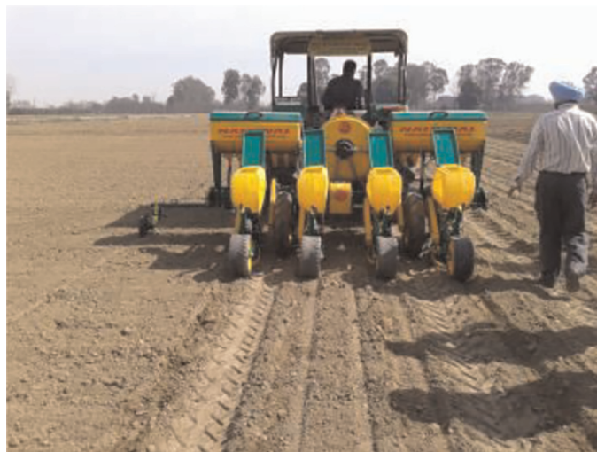
Figure 14. Maize sowing with pneumatic flat planter during 2017.
