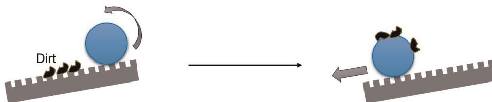
Figure 3. Schematic representation for the mechanism of self-cleaning from a super-hydrophobic surface.
