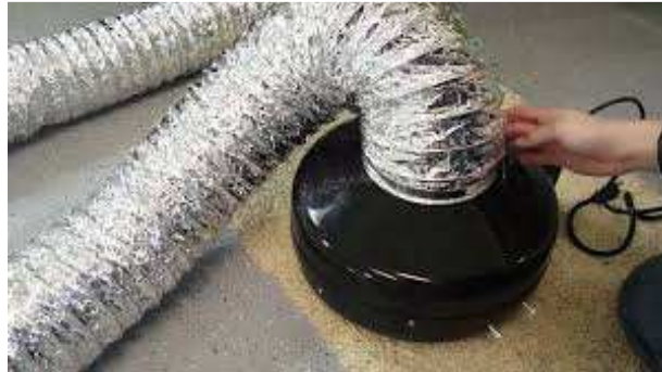
Figure 9: Fume hood used to exhaust evaporated solvent and nanoparticles which do not attach to collector.
