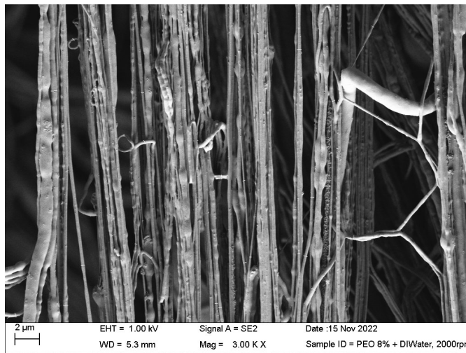
Figure 14: 3000X Magnification 8 wt% PEO in DI H2O at 2000 rpm and 2000V
