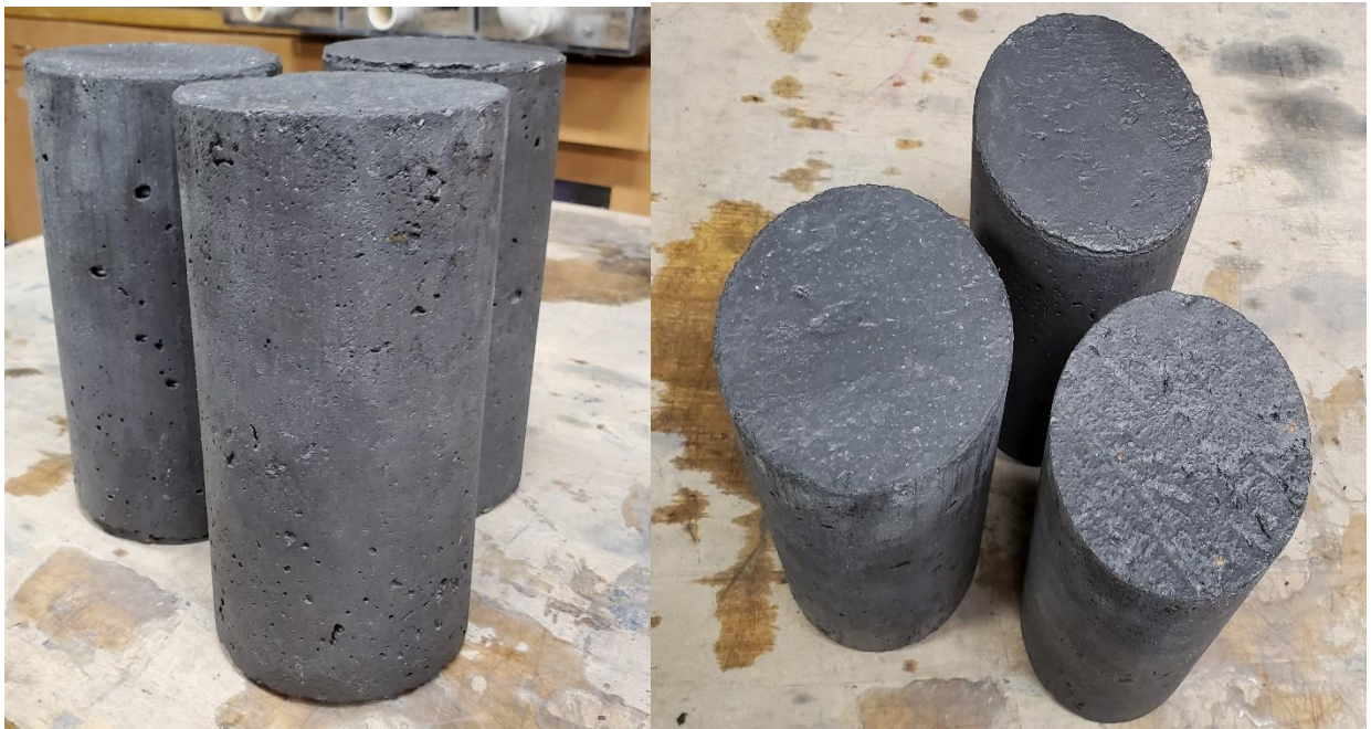
Figure 8: Conductive concrete cylinders containing 10% graphite by volume. Specimens are 10 cm by diameter and 20 cm by length. (a) side view of the specimens and (b) top view of the cylindrical specimens.
