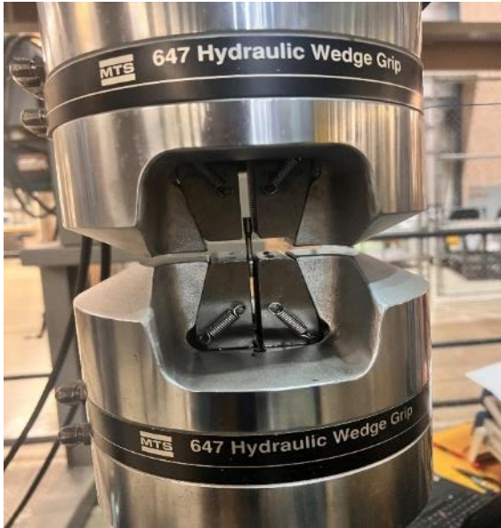
Figure 3: Sample set up in the fatigue testing machine
