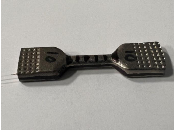
Figure 7 : Sample specimen with marking for cutting
