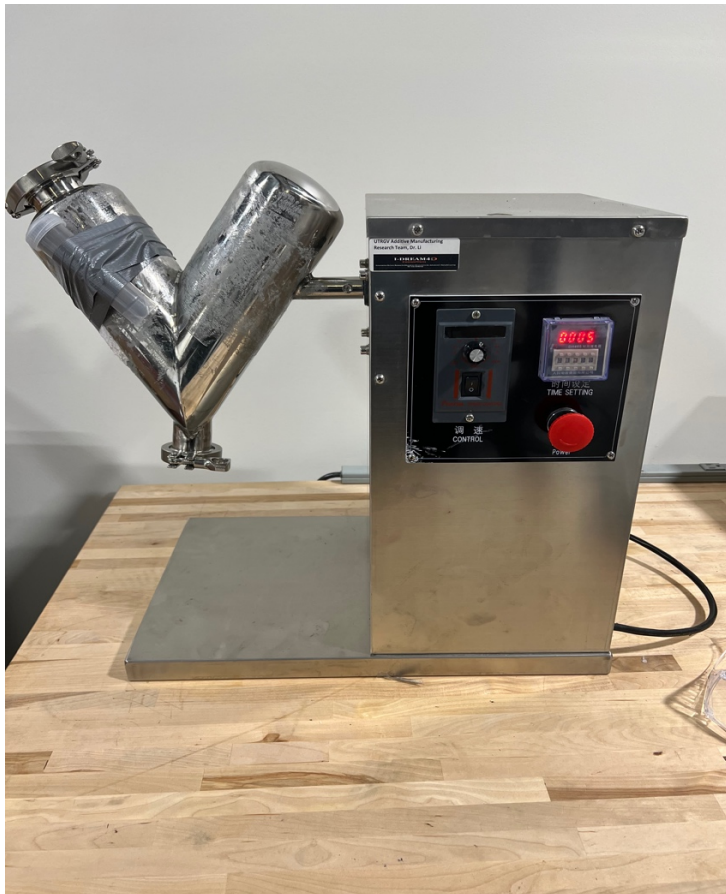
Figure 5: V-Type Blender to mix the powder.
