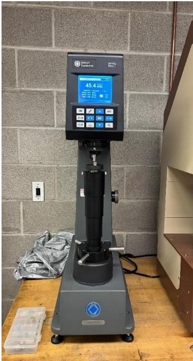
Figure 14: Wilson Hardness Rockwell 574 tester
