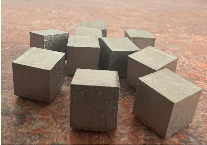
Figure 5: SLM printed Inconel 718 samples
