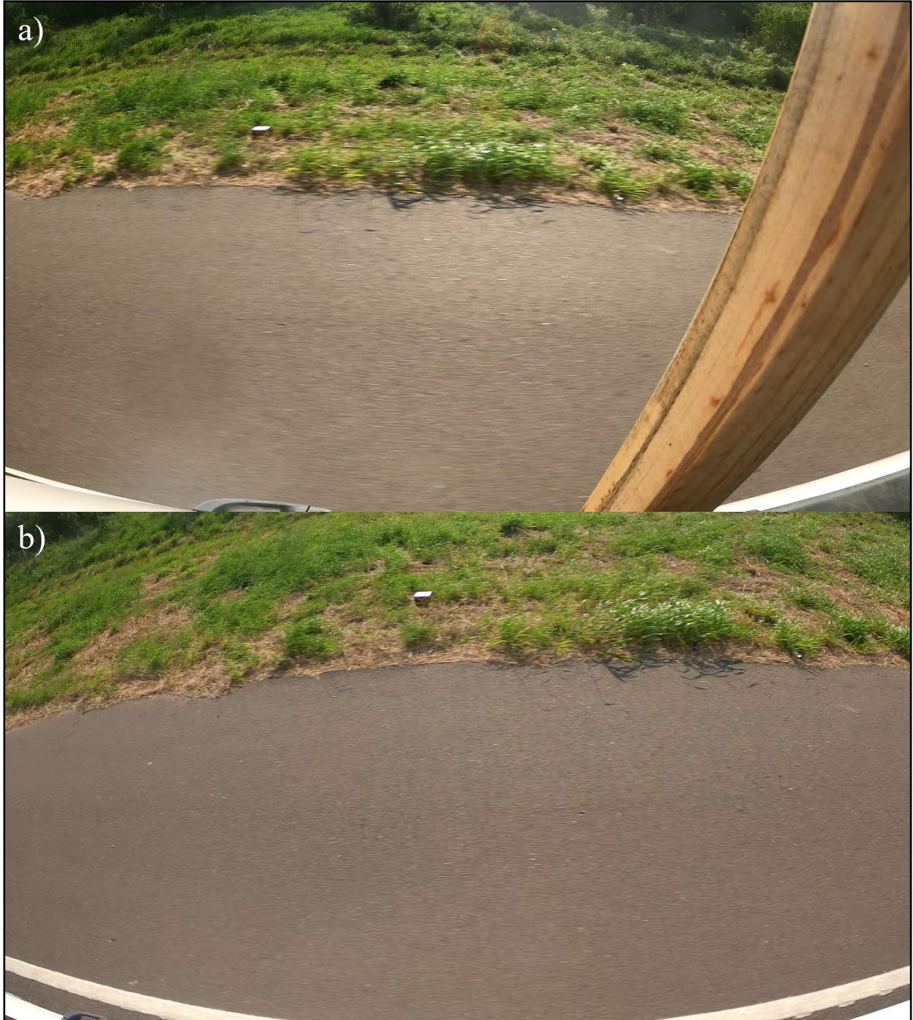
Figure 13. Field of view (FOV) comparison of camera positions 6a (a) and 7a (b). Weighted cardboard boxes with Snellen eye charts are the targets of these screenshots. Position 7a provides more top-down coverage. Positions 6a and 7a provided the best 2 right-facing FOV.
