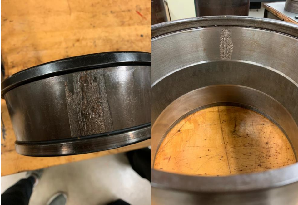
Figure 2: Cone spall (left) and Cup spall (right)
