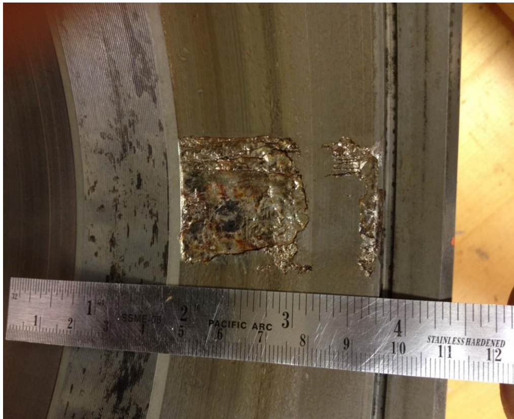
Figure 15: Picture of spall on B2 bearing cup from experiment 200
