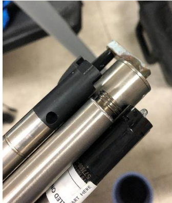
Figure 14. Sensors contained in the YSI EXO2 Sonde and the automatic wiper at the top
