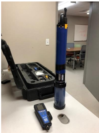
Figure 13. YSI EXO 2 sonde along with the handheld that stores data and their hard case.
