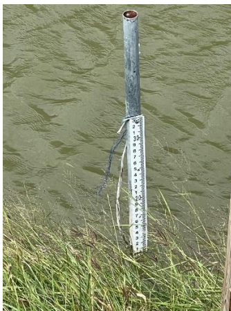
Figure 21. Staff gage installed at Station 22120.
