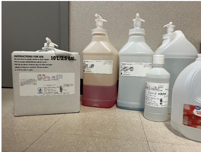
Figure 15. Calibration standards: pH 7, pH 4, pH 10 (two 10L bottles), conductivity 10,000 uS/cm, and distilled water (from right to left).
