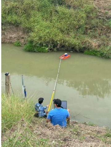
Figure 20. Discharge measurement using the ADCP.
