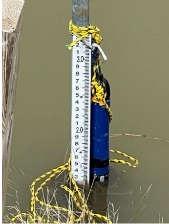
Figure 17. YSI EXO2 Sonde installed at station 22118.
