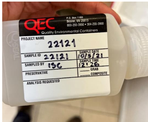
Figure 23. Sterile plastic container with a capacity of 250 ml provided by Ana-Lab to assess bacteria concentration.
