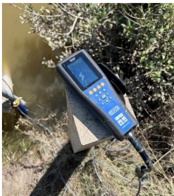
Figure 18. Handheld connected to YSI EXO2 sonde to store water quality data from Old Main Drain Ditch.
