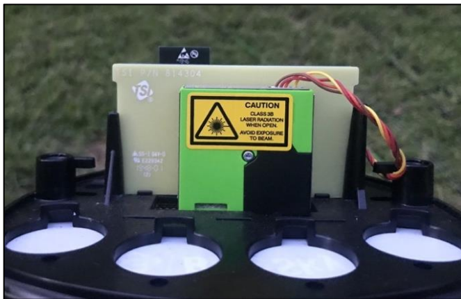
Figure 3.19: Photo of the installed PM sensor.
