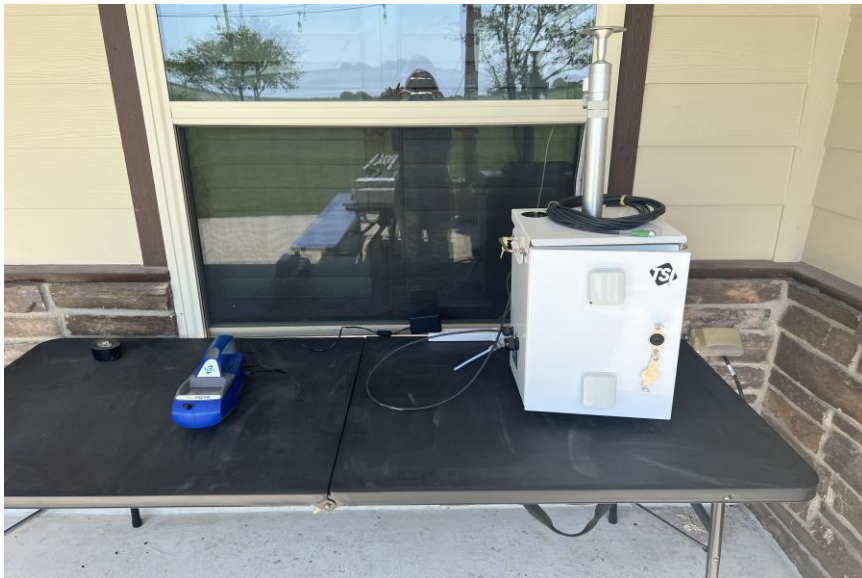
Figure 4.12: Installation photo of FEM1 DustTrak Environmental Monitor with FEM2 DRX Aerosol Monitor.
