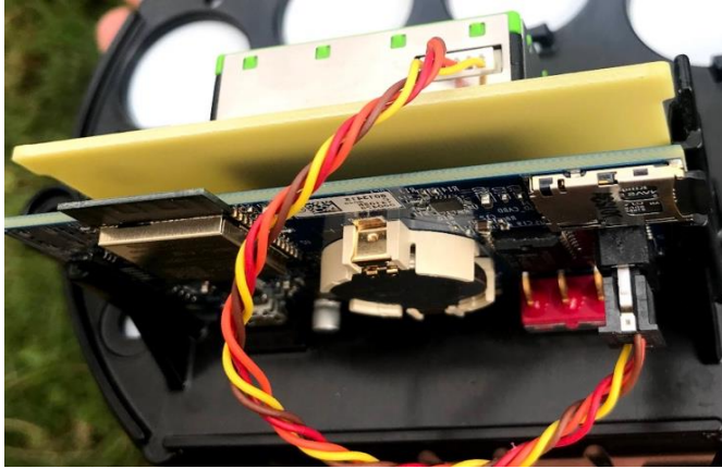
Figure 3.21: Top profile of the installed PM sensor.
