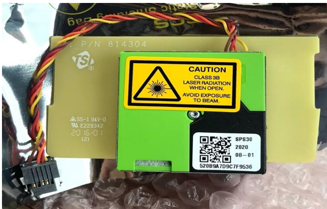
Figure 3.22: Uninstalled PM sensor.
