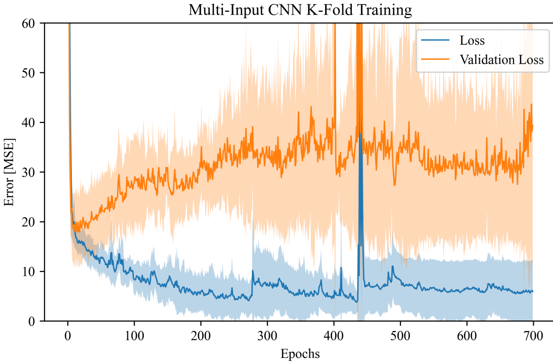
Figure 3.9. Multi-input CNN produces noisy loss, unlike the multi-input MPNN model.
