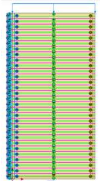
Figure 3.1: Geometry generation of a L/H 05. Wall with a reinforcement spacing of 0.2m.
