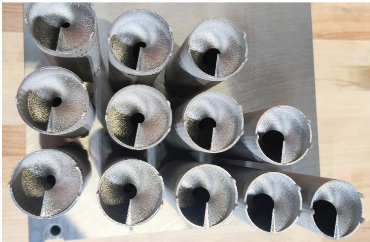
Figure 30: Solar absorber tube with internal fin structure
