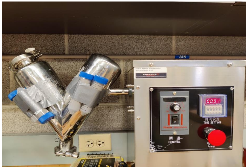
Figure 19: B with IN718 powder mixing in the V-shape mixture
