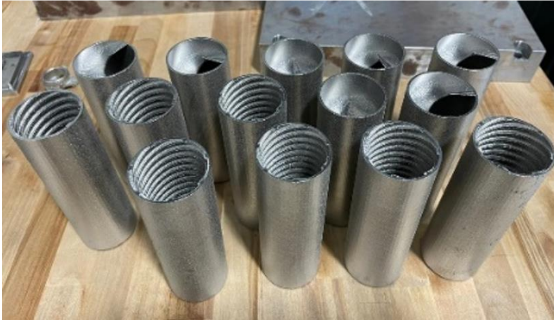
Figure 16: larger section of the tubes with multi-head and continuous helical fins
