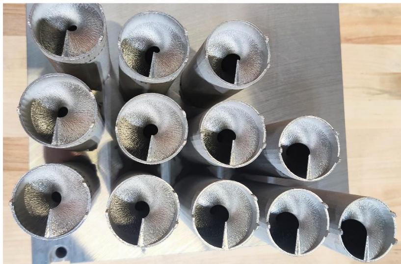
Figure 15: Larger section of tubes with Continuous helical fin structure
