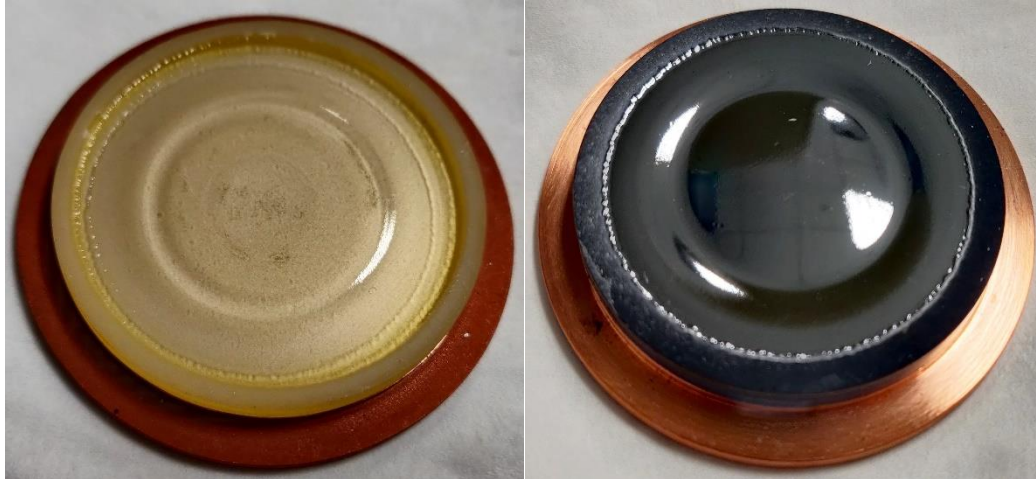
Figure 2.4: SiO 2 (left) and pSi (right) target used for sputtering
