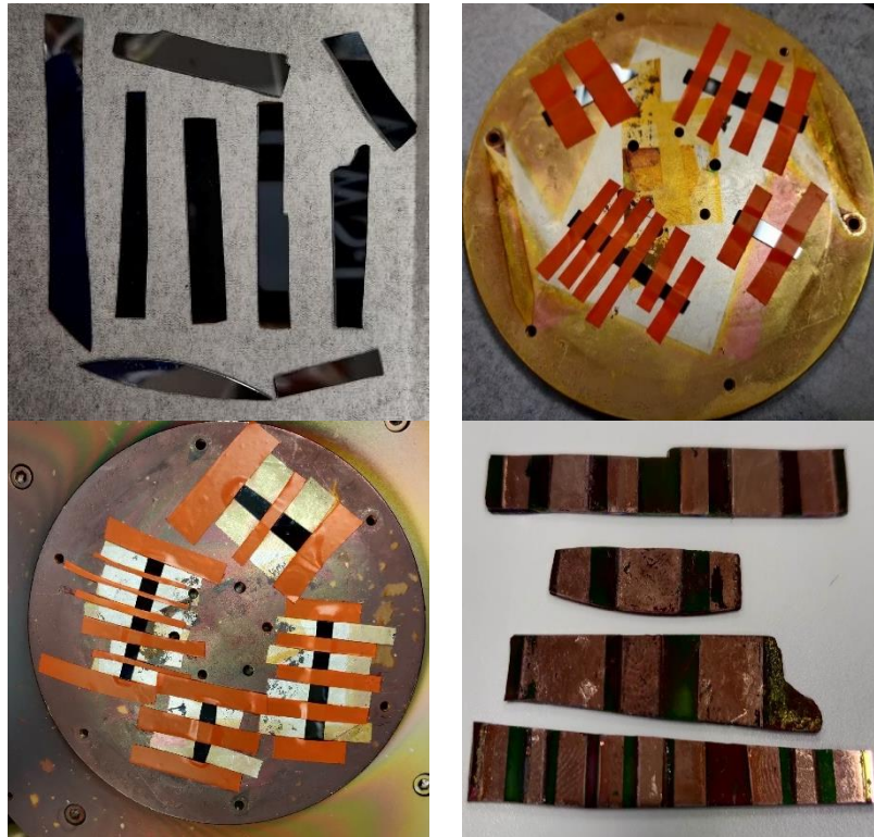
Figure 5.2: Steps of n-MOSFET Fabrication. Si sample substrate (topleft), p-Si overlayers deposition and channel length (topright), n-well deposition and length (bottomleft) and final n-MOSFET samples with Cu contact layers (bottom right)
