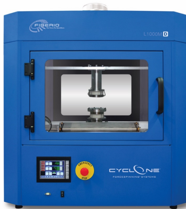
Figure 25. FibeRio's cyclone L-1000 Forcespinning® machine [52]
