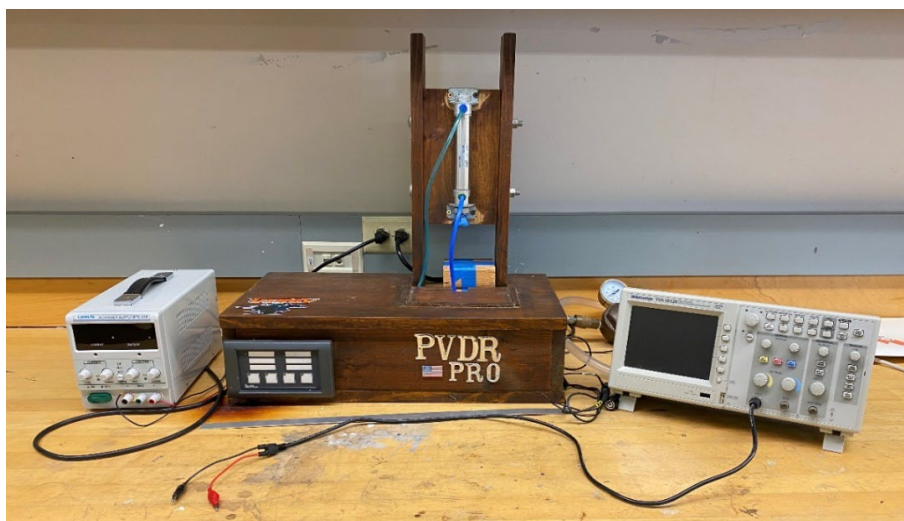
Figure 38. PVDR PRO and Tektronix TDS 2012B oscilloscope for piezoelectric response
