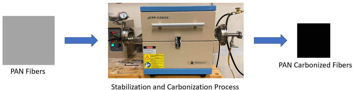
Figure 31. Stabilization and carbonization process for PAN fibers
