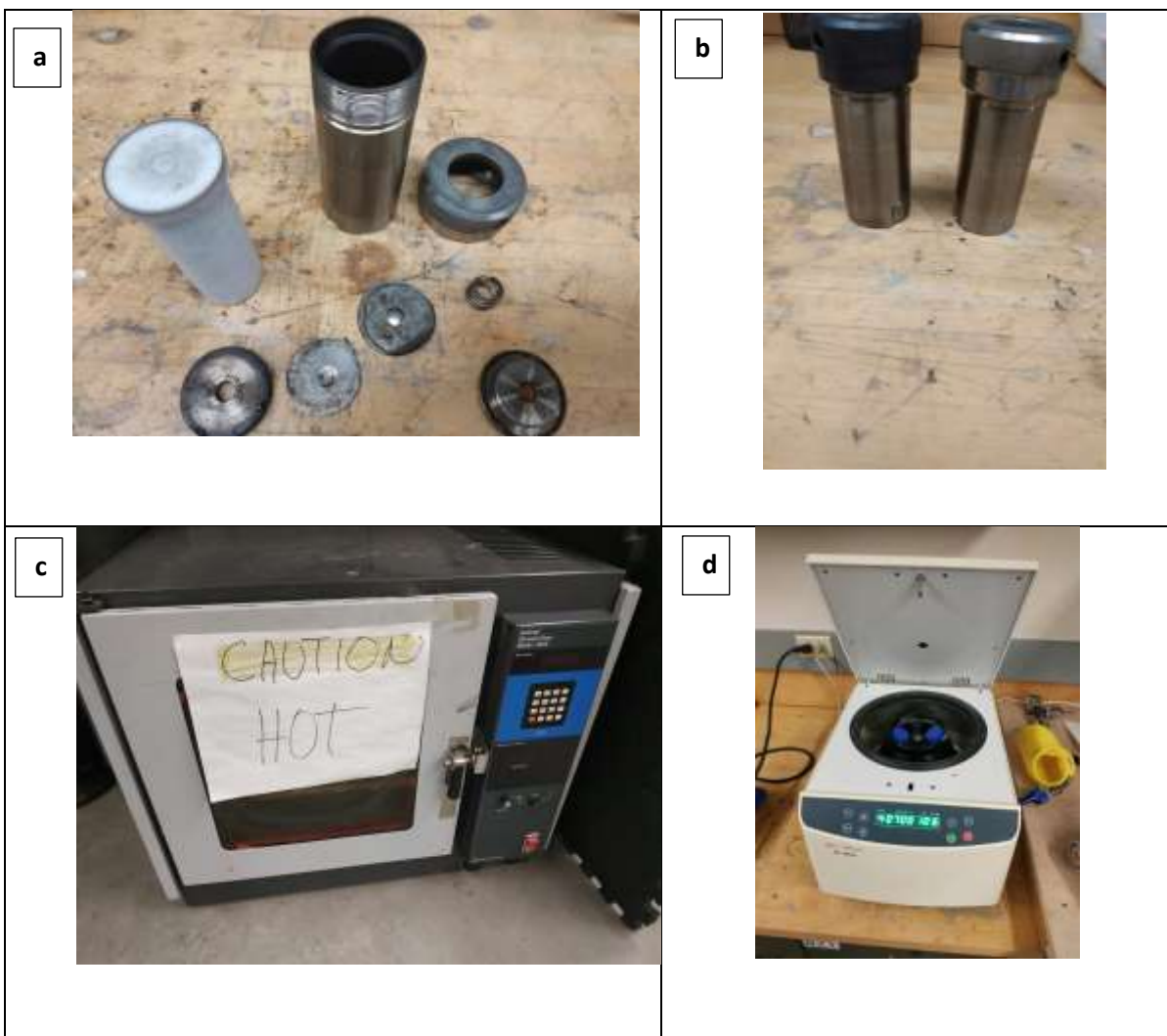
Fig 12: a) Hydrothermal Reactor parts b) Hydrothermal Reactor c) Oven d) Centrifuge m/c
