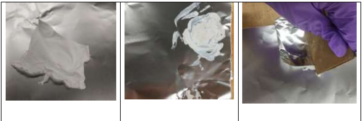
Fig 13: Fiber mat submerged into Water-DMF-Nanoparticle Solution
