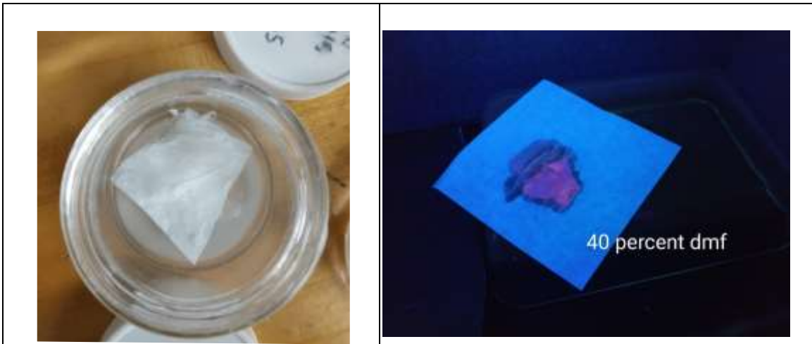
Fig 13: Fiber mat submerged into Water-DMF-Nanoparticle Solution
