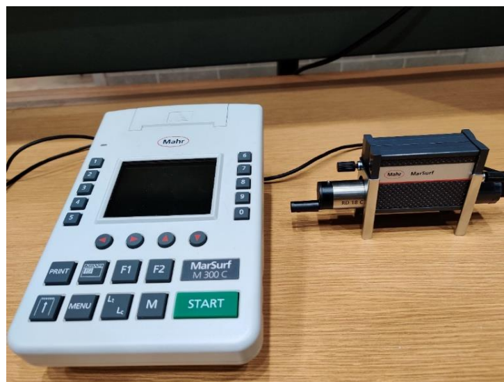
Figure 6: Surface roughness measurement set up using MahrSurf M 300 C profilometer
