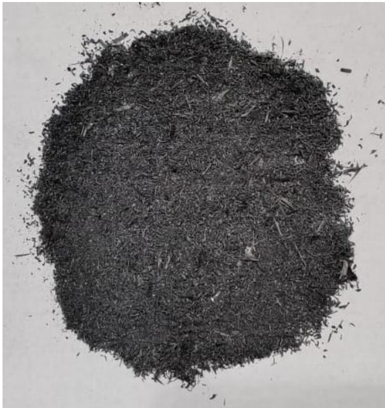
Figure 31: Powder like chips produced during turning process of CFRP
