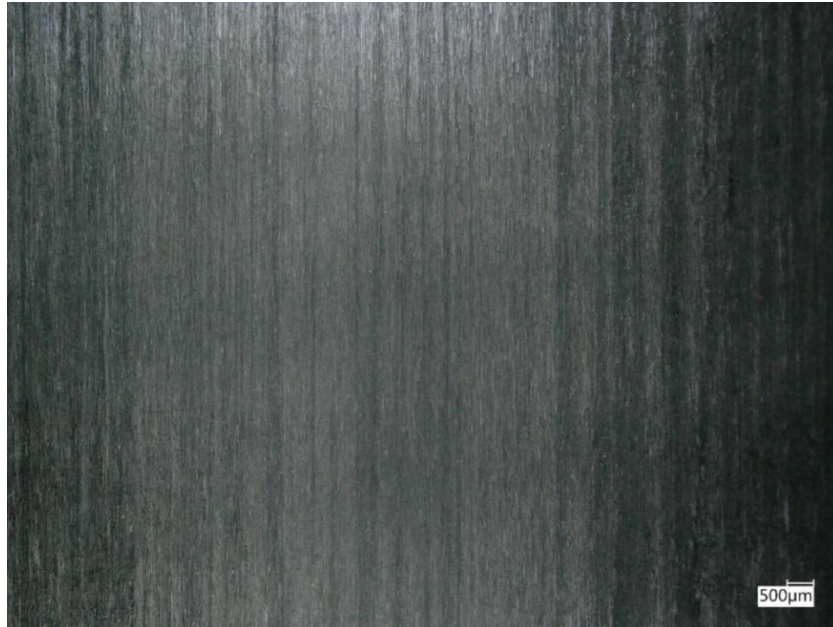
Figure 15: Optical microscopic view of machined surface obtained at cutting speed of 100 m/min, feed rate of 0.05 mm/rev and depth of cut 0.15 mm
