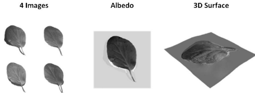
Figure 6: Four Images Acquired Using Different Lighting Sources, an Albedo Image, and a 3D Reconstruction
