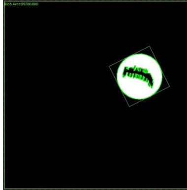
Figure 20: Trial 22- Wafer with Large Marker Blob (Predicted and Tested)
