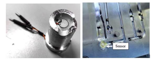
Figure 5: Installed Piezo disk inside mold
