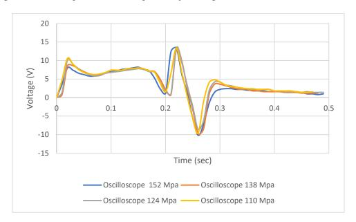
Figure 18: Voltage reading for different machine injection pressure Another consideration is the calculated pressure conversion coefficient is based on Mold flow estimation, not from an actual pressure measurement. It is suggested that installing a calibrated conventional pressure transducer for actual pressure reading to calculate accurate pressure conversion factor.
