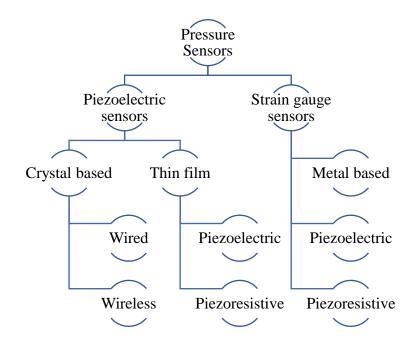
Figure 1: Classification of Pressure Sensors (Ageyeva et al., 2019)
