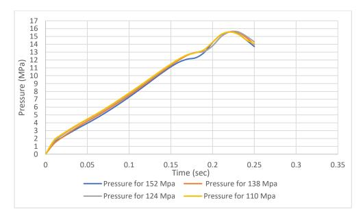
Figure 16: Cavity Pressure Profile from Oscilloscope data
