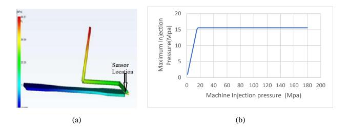
Figure 11: Pressure profile from Mold Flow simulation
