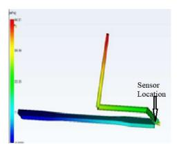
Figure 4: Product specimen from mold flow simulation
