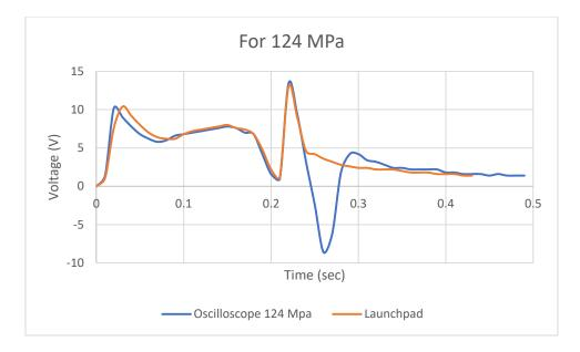
Figure 14: Voltage reading from Sensor when machine injection pressure was 124 MPa
