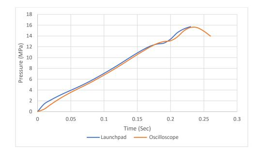
Figure 15: Cavity Pressure Profile when machine injection pressure was 138 MPa
