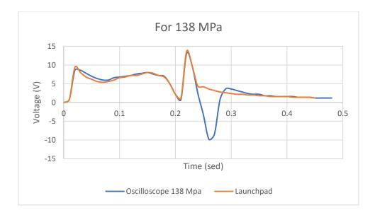
Figure 12: Voltage reading from Sensor when machine injection pressure was 138 MPa
