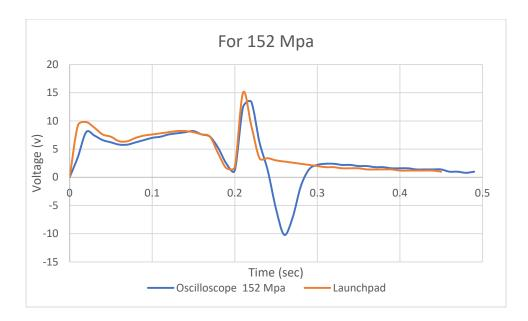
Figure 13: Voltage reading from Sensor when machine injection pressure was 152 MPa
