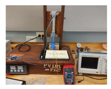
Figure 9: Pneumatic punch machine for generating pressure
