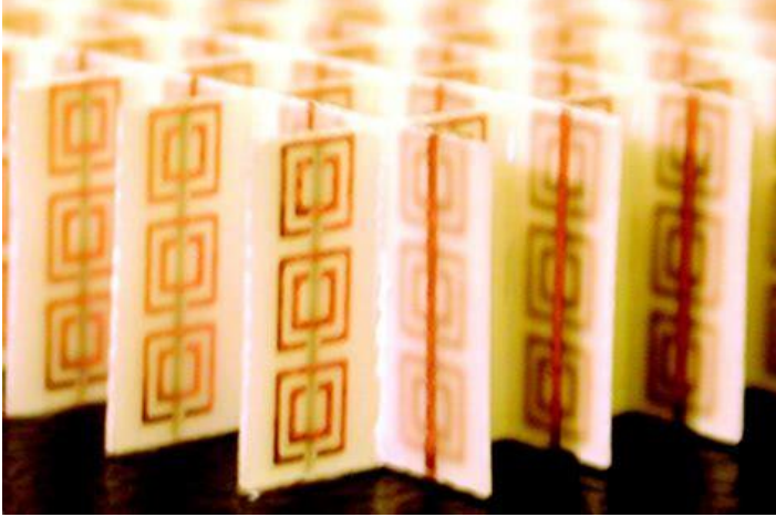
Figure 1.4: Construction of Metamaterial with Copper Strips and Split Rings [7]
