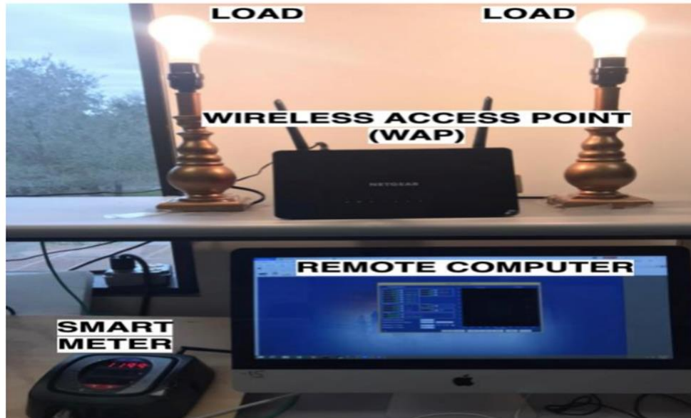
Figure 2.5: Lab setup used in experiment showing Load, Smart meter and remote monitoring computer.
