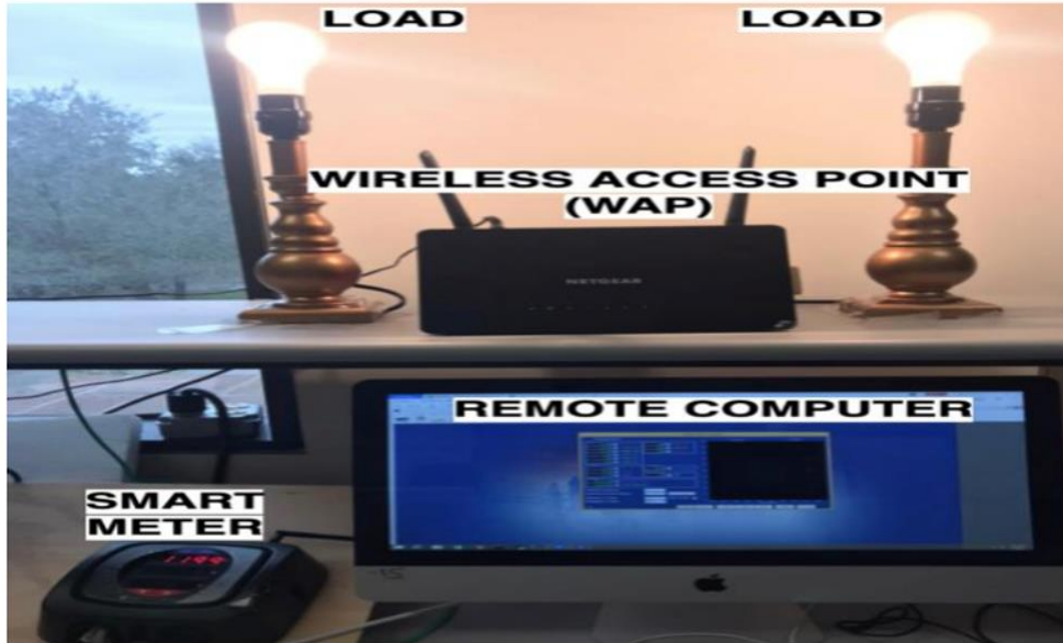
Figure 3.3: Lab setup used in experiment showing Load, Smart meter and remote monitoring computer.
