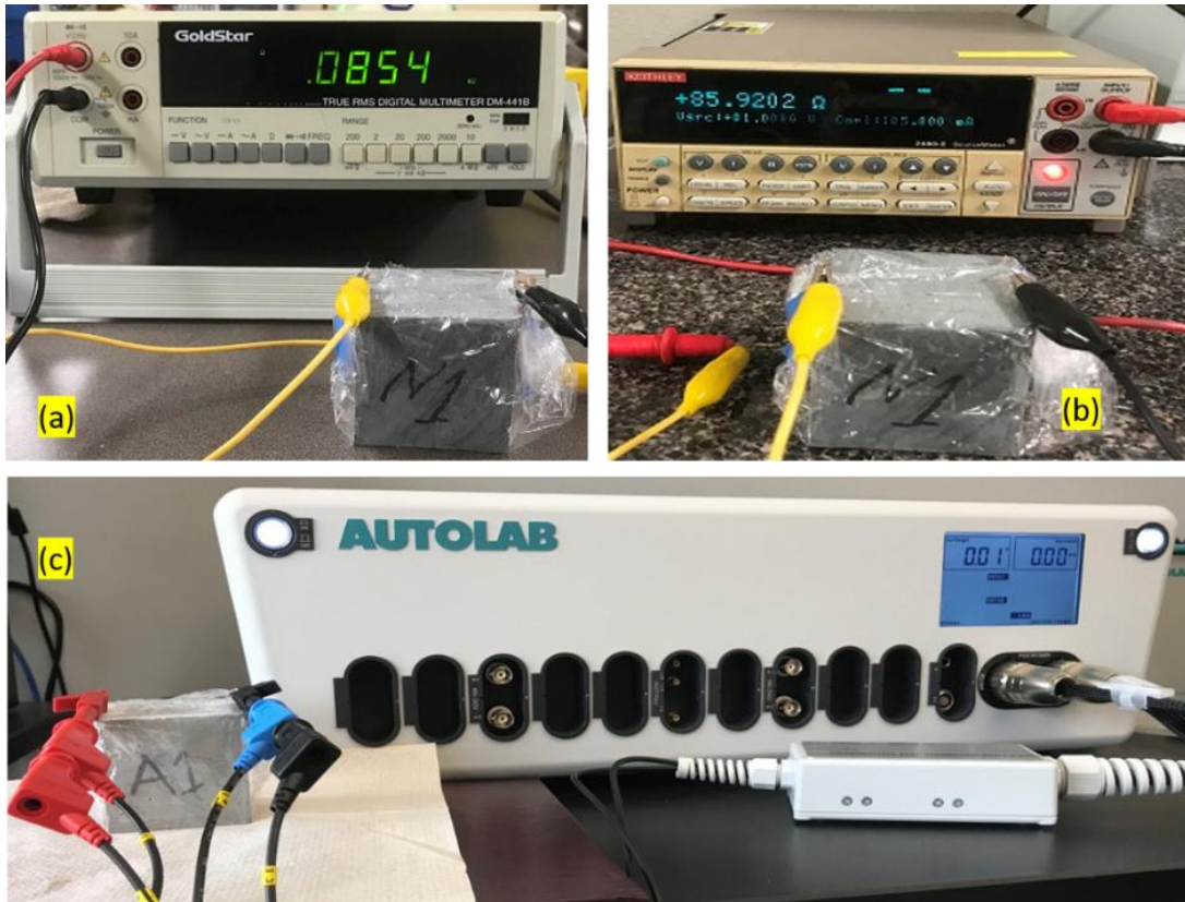
Figure 3.2: Test Set up for measuring static (DC) resistance through (a) True RMS Digital Multimeter DM-441B (Multimeter-2) (b) Keithley 2400 (C-22) Source Meter (Multimeter-1), and for AC Impedance measurement through (c) Metrohom AUTOLAB PGSTAT302N
