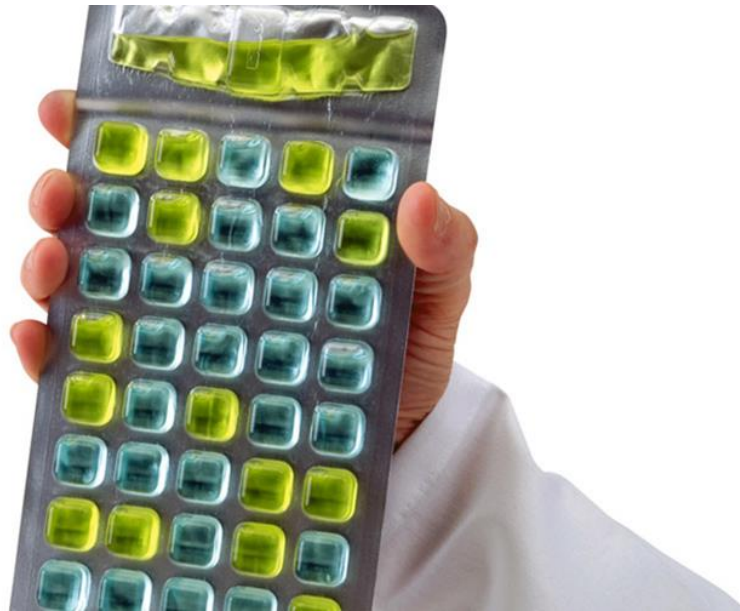
Figure 8. IDEXX Quanti-Tray. Quanti tray system uses nutrient indicators to quantify coliform and E. coli .
