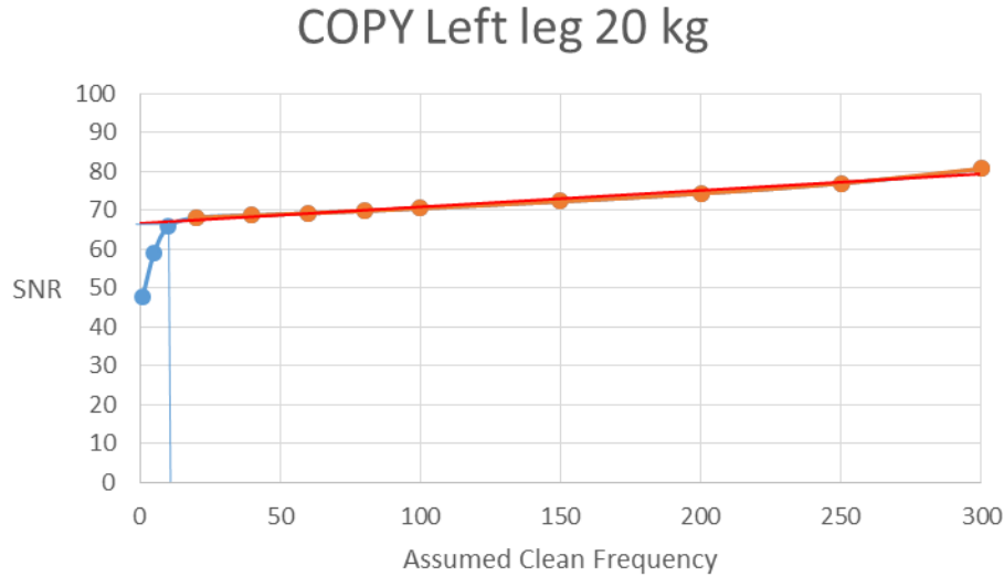
Figure 108 SNR vs Assumed Clean Frequency Center of Pressure Y of left leg with 20 additional weight.
