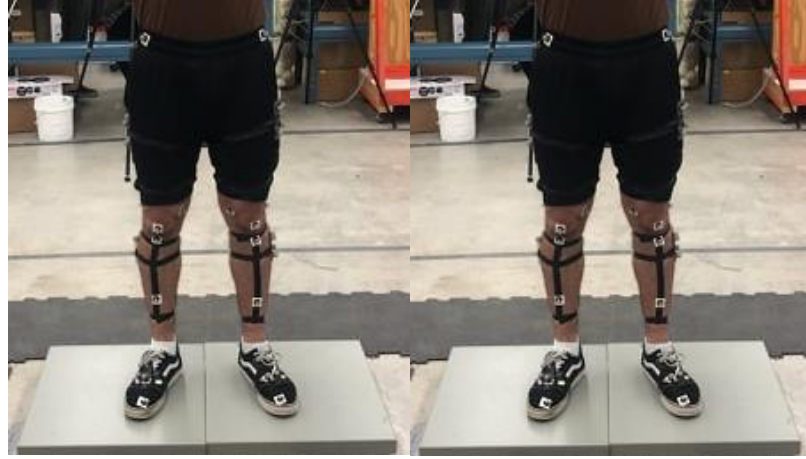
Figure 7 Subject on the force Plates.
