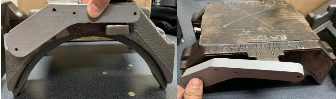
Figure 17: Fit test on Class K steel adapters; left (new design) and right (old design)
