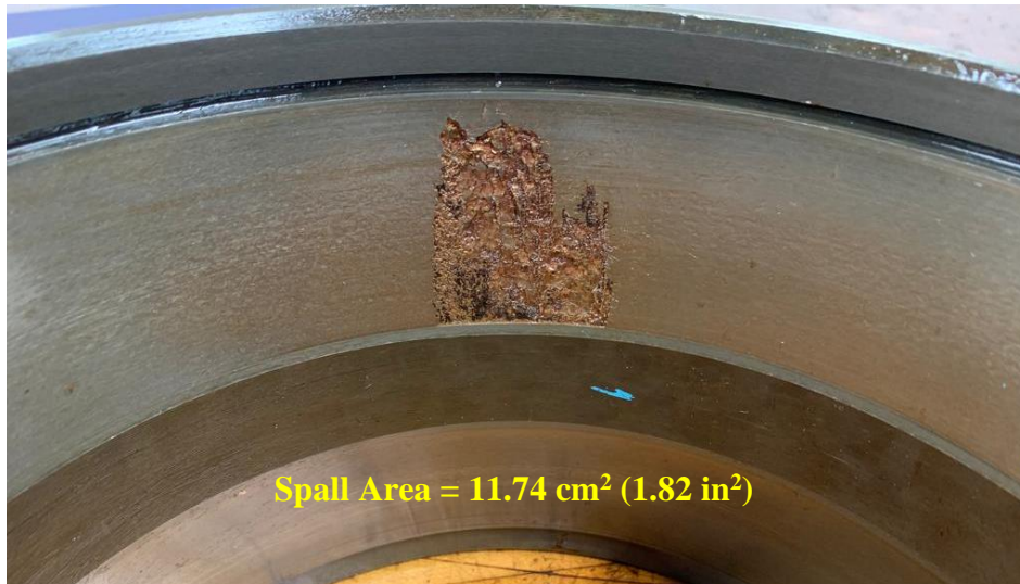
Figure 35: Experiment 231 B3 – medium-size cup spall
