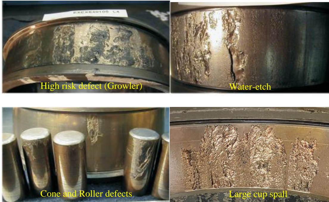
Figure 2: Tapered-roller bearing defects
