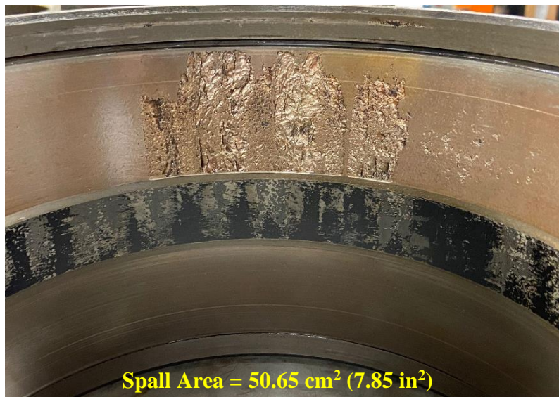
Figure 38: Large cup (outer ring) spall used in Experiment 232 for validation testing of Boomerang B
