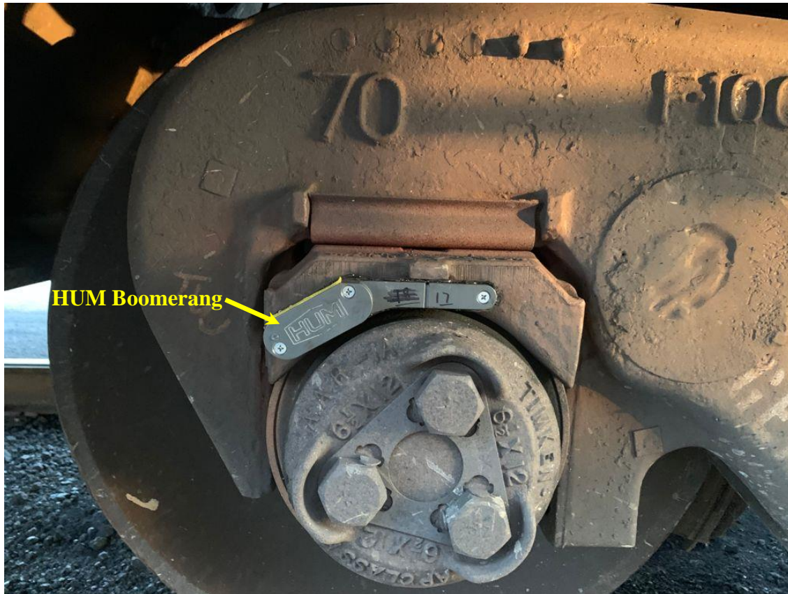
Figure 24 : Boomerang B field installation
