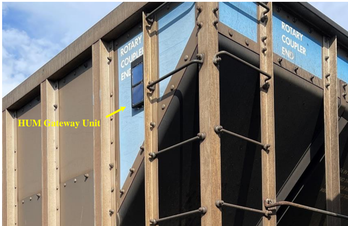
Figure 23 : Gateway field installation on a freight railcar
