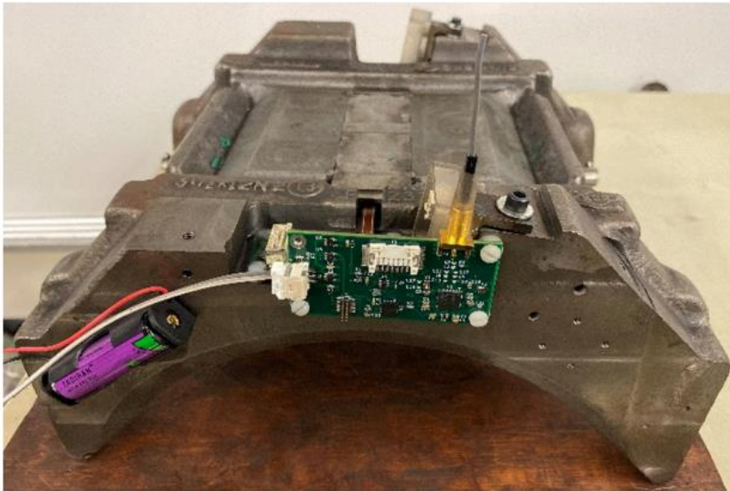
Figure 9: UTCRS wireless onboard condition monitoring module and power source [28].
