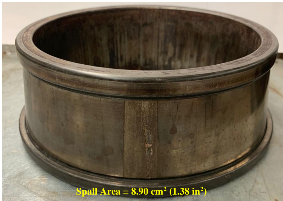
Figure 41: Experiment 233 cone defect tested in B3 position
