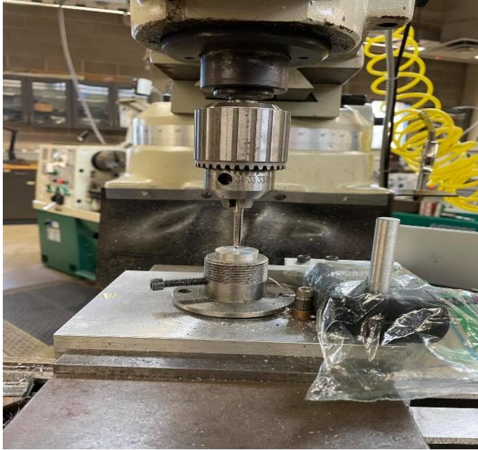
Figure 11 : Tapping torque test in Grizzly milling machine.
