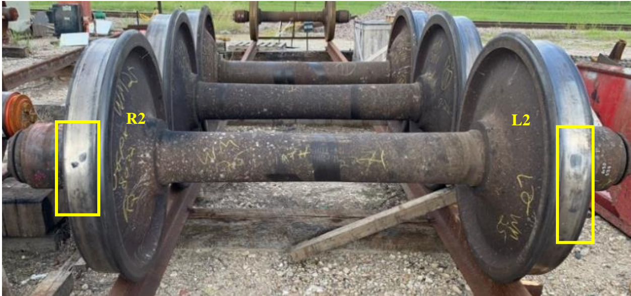
Figure 33. Axle 2 high-concern wheelset (defective)
