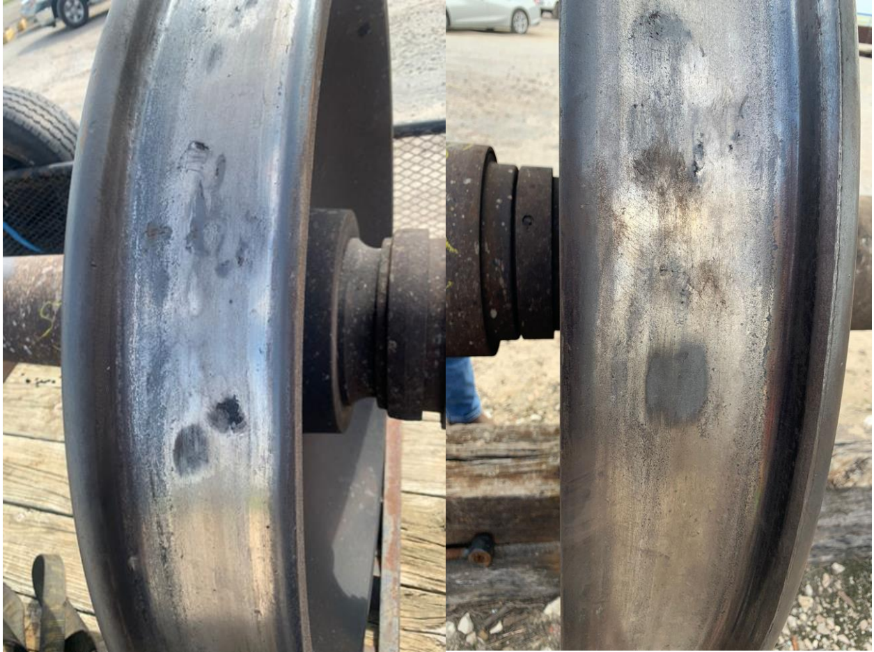
Figure 52. Defective Axle 2: wheel R2 defects (left) and wheel L2 defects (right)
