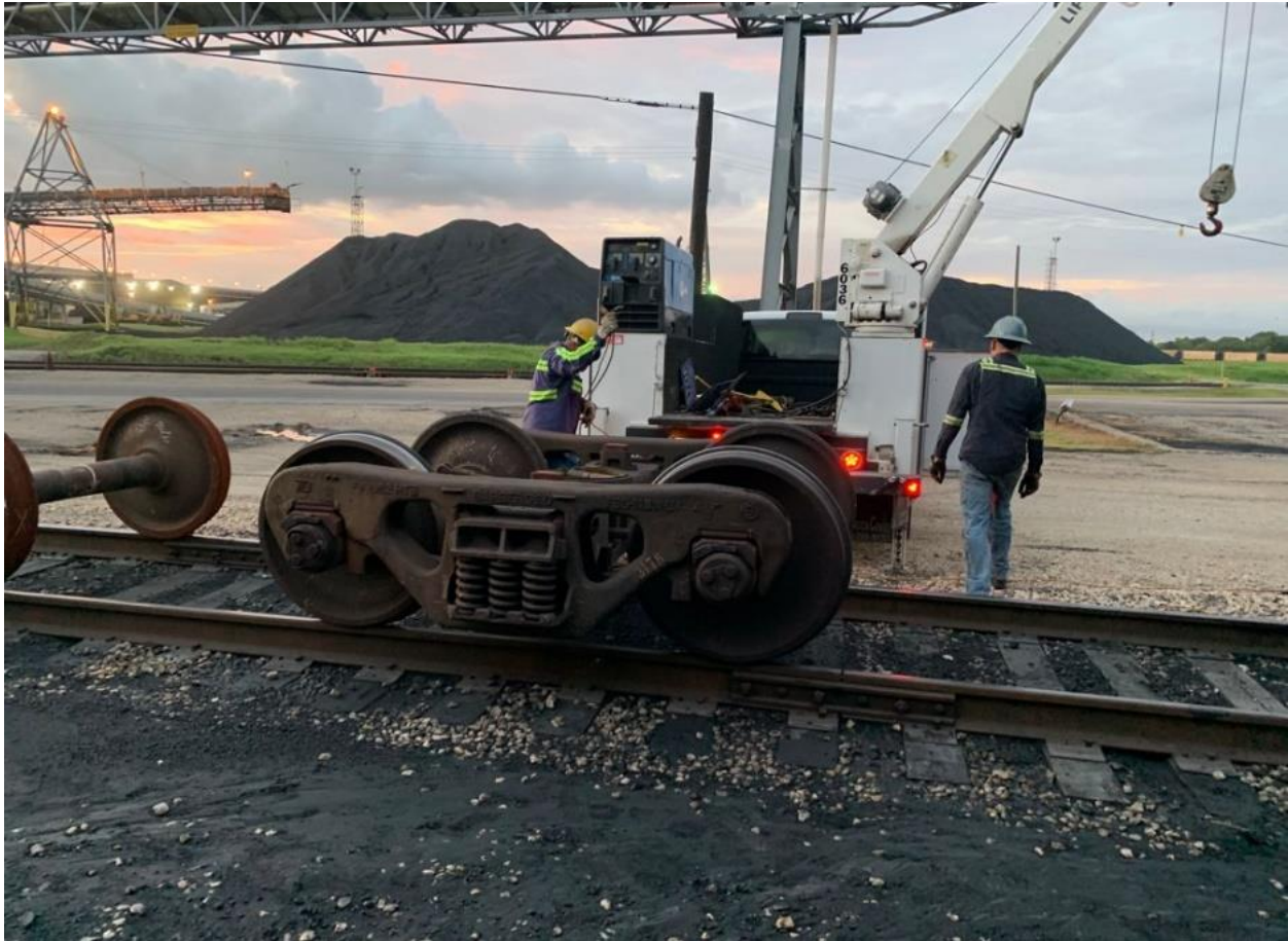
Figure 31. Wheelset removal process
