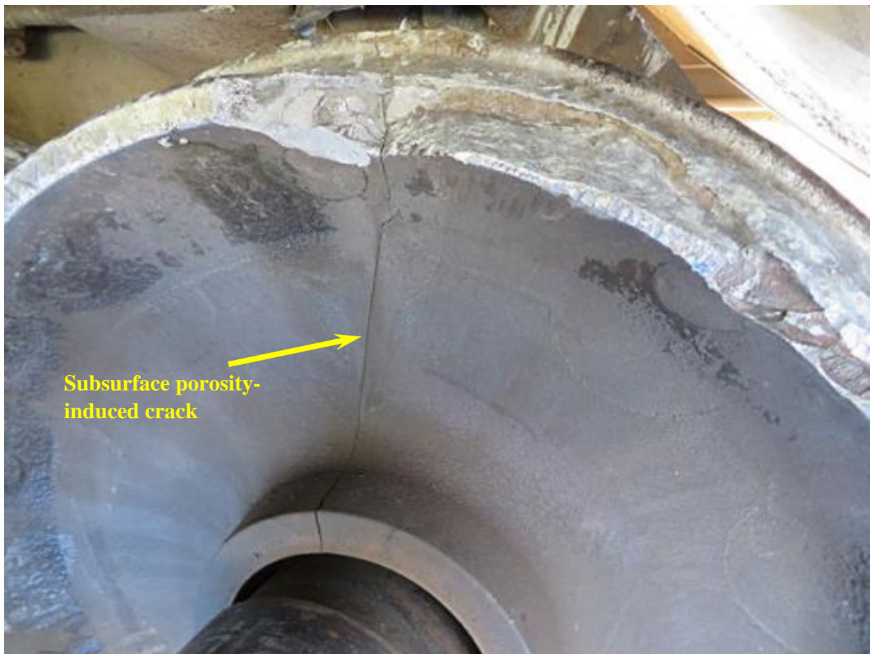
Figure 7. Cracked wheel L3 of railcar CRDX 15109 [27]
