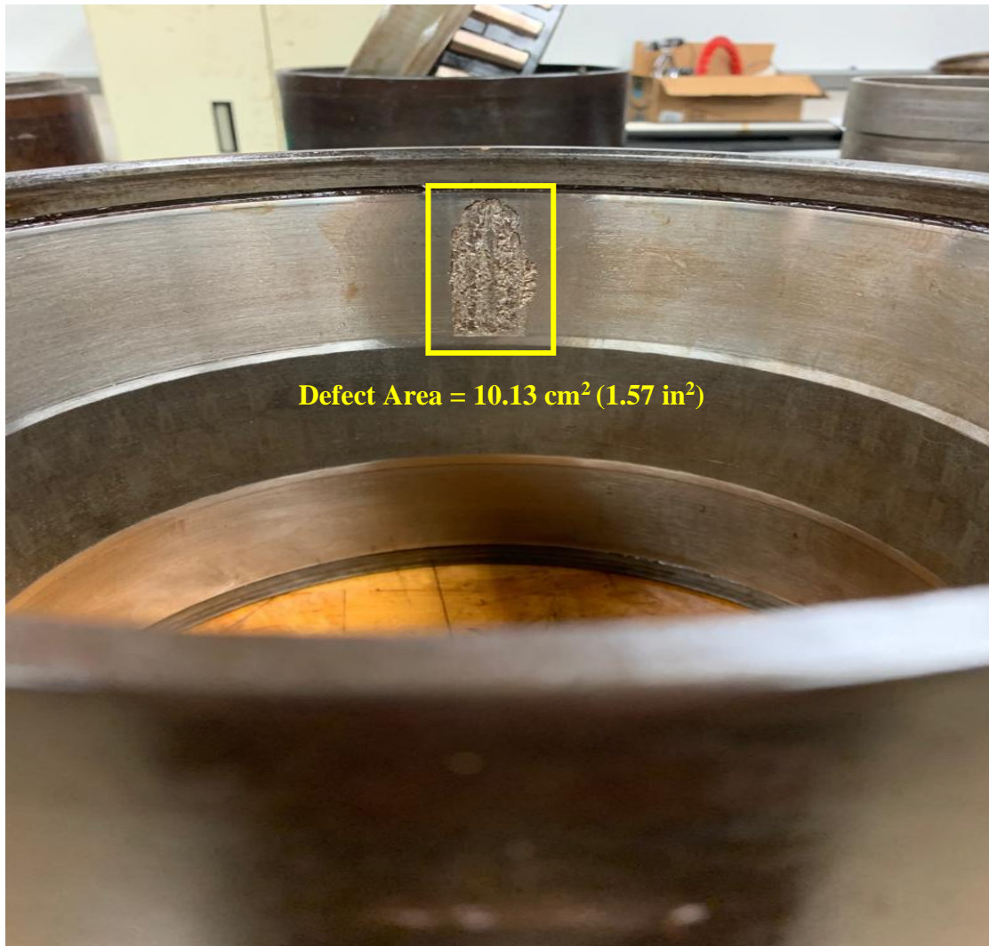
Figure 39. Experiment 246 cup containing a raceway spall of 10.13 cm 2 (1.57 in 2 )
