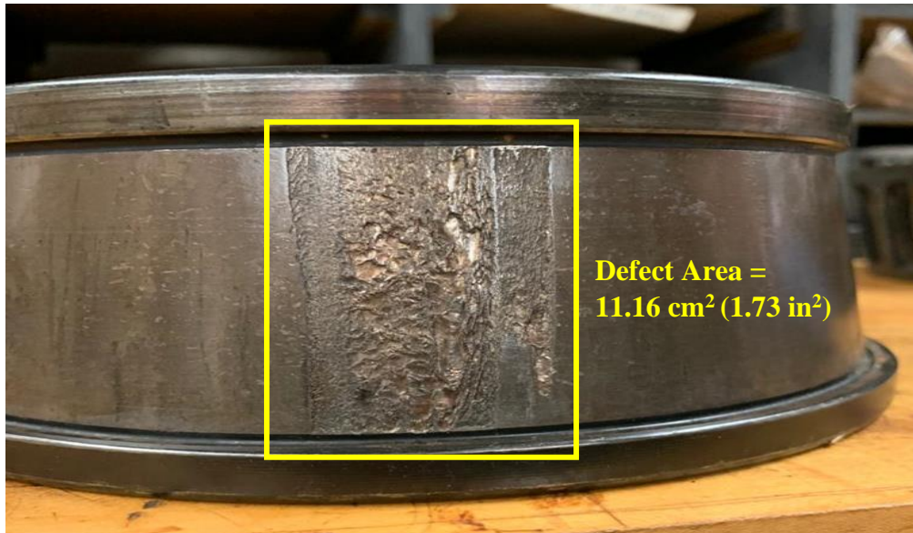
Figure 36. Experiment 245 cone containing a raceway spall of 11.16 cm 2 (1.73 in 2 )
