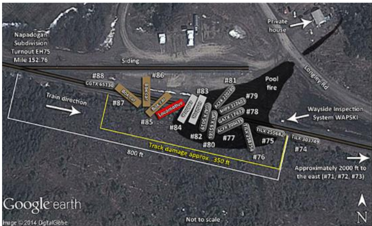
Figure 6. Diagram of freight train M30831-06 derailment [27]
