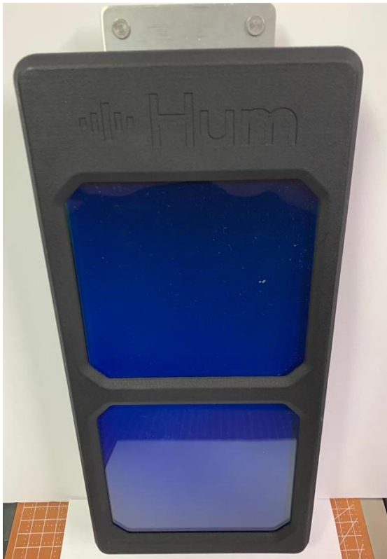
Figure 18. HUM central communication unit (i.e., Gateway)
