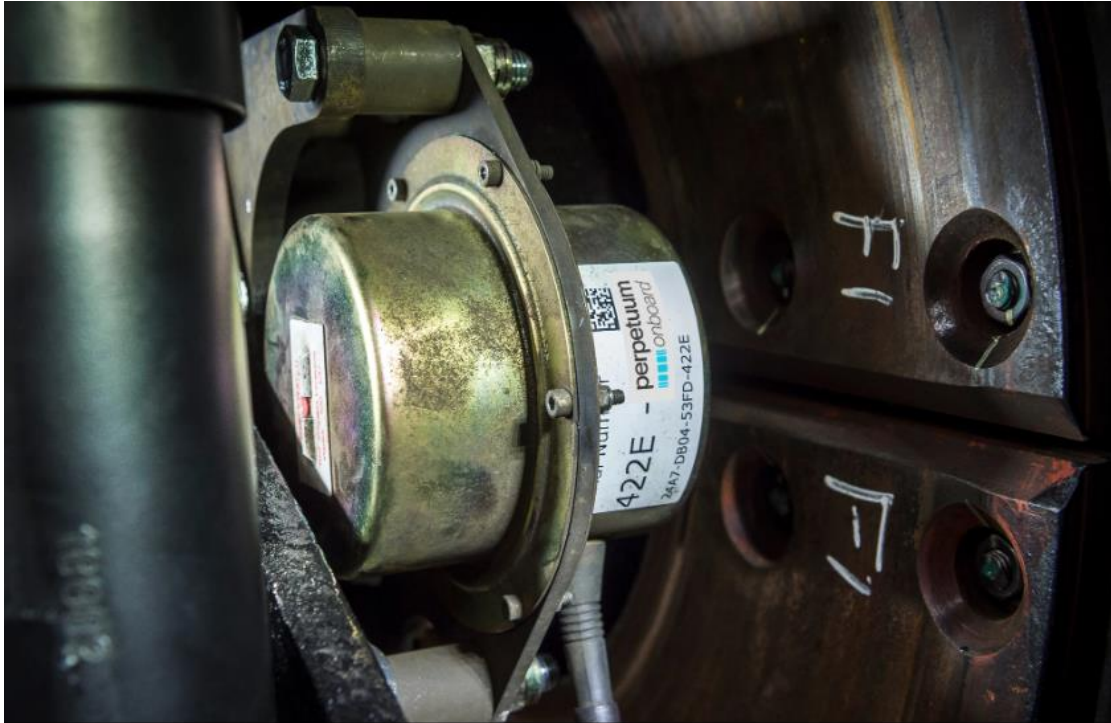
Figure 15. Perpetuum system mounted on railcar wheel hub [46]
