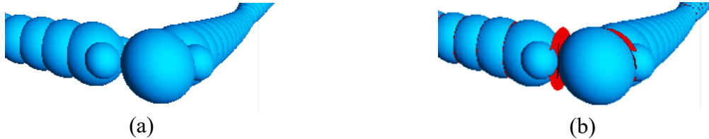
Figure 3. (a) geogrid consists of strings of overlapping bonded spherical balls, (b) parallel bonds (red)
