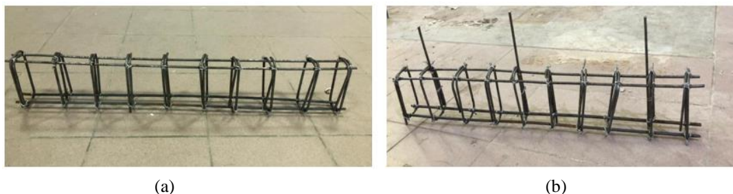
Fig.2: Beam reinforcement details; (a) for beams in normal condition and (b) for beams exposed to accelerated corrosion.
