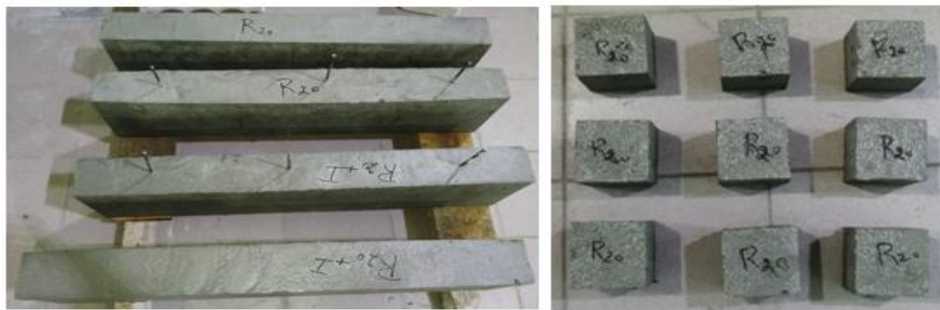
Fig.3: Casted beams and cubes
