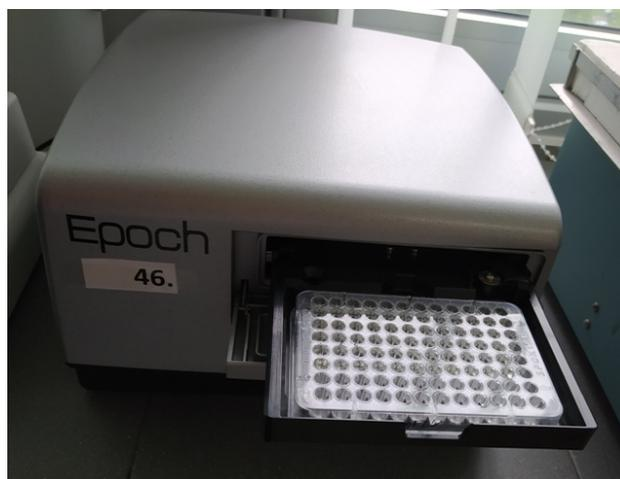
Figure 4. Reading of results by BioTek Epoch type spectrophotometer (Photo: G. Barać)
