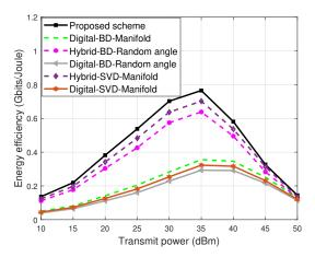
Fig. 9. Energy efficiency versus the transmit power of the BS.
