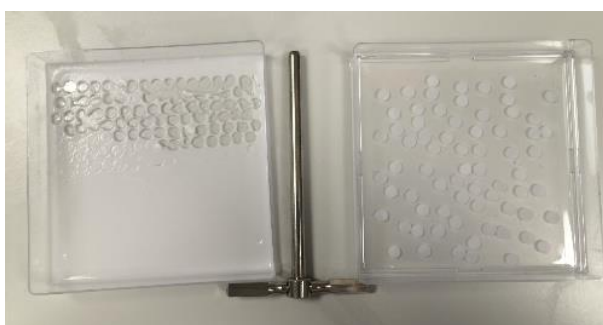
Figure 2.2. Disc production from polymer A. Image shows polymer A cast into a 100 mm (width) x 100 mm (length) x 20 mm (depth) square petri dish - left. The cork borer used to cut discs from the polymer sheet – centre. Resultant 6 mm diameter polymer A discs – right.
