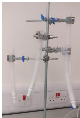
Figure 2.3. Polymer A cast into a 15 mm diameter cylindrical format using silicon tubing. Image shows sections of silicon tubing plugged with a tubing connector, suspended vertically using a clamp stand, and partially filled with polymer A solution.
