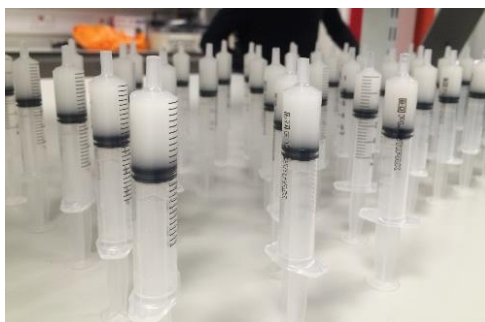
Figure 2.1. Polymer A cast into a cylindrical format using a syringe. Image shows 2 mL of polymer solution taken into a 5 mL syringe.
