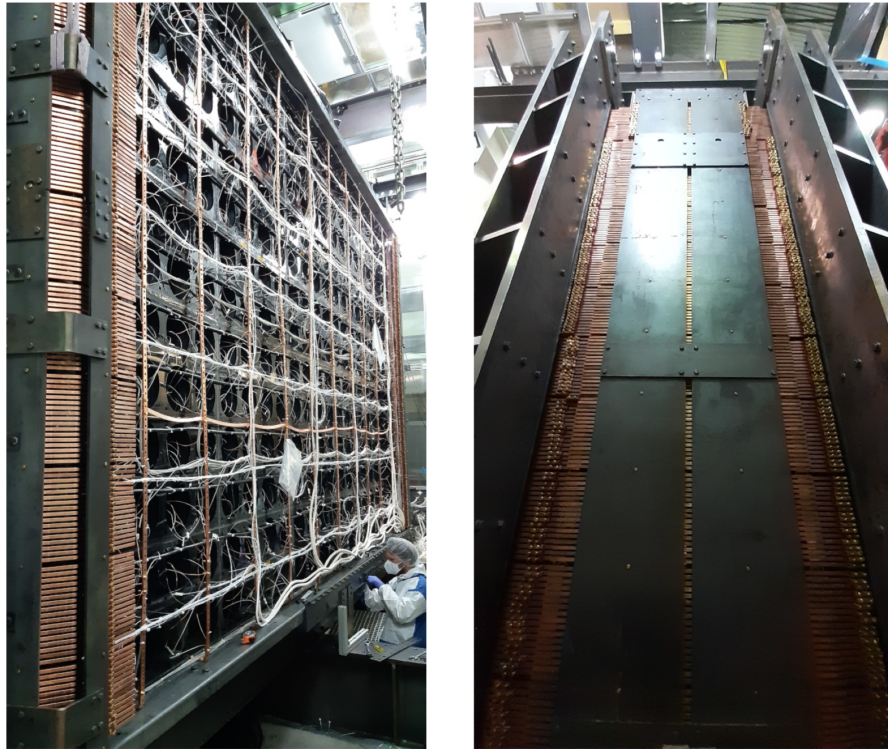
Figure 5.6: Image of the installation of the copper coil to provide a uniform magnetic field in the detector. (Left) The installed copper field wrapping around the calorimeter wall. (Right) The side on view of the detector where the source is central, surrounded by the tracker sections and finally the calorimeter walls [83].
