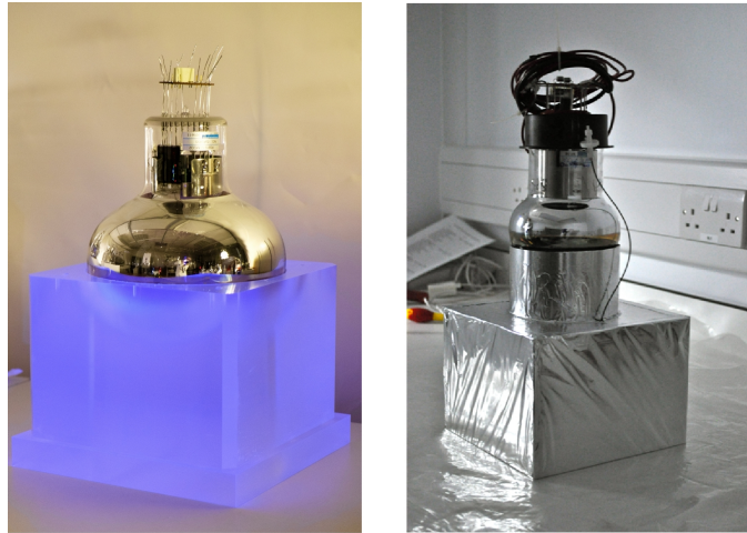
Figure 5.5: (left) 8" PMT directly coupled to polystyrene scintillator block and (right) a 5" PMT coupled via a light guide
