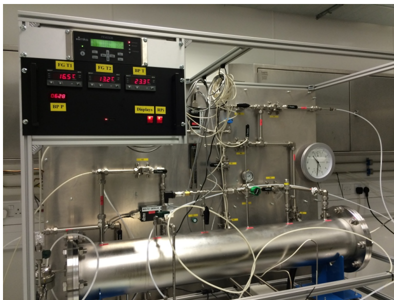
Figure 7.9: Photo of the final crate location, at the top left of the gas system rig, with the PR4000B-F MFC secured on top.
