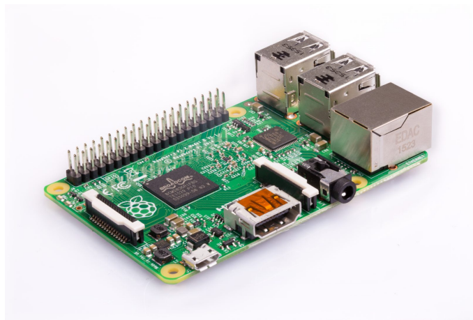
Figure 7.4: Photo of the Raspberry-Pi 2 Model B [120] .
