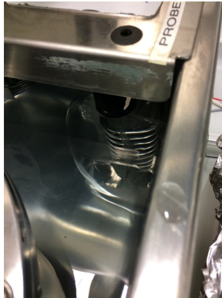
Figure 7.15: Ice forming on the cooling element of the EK20 unit at a temperature of \approx 2^\circ\text{C} .
