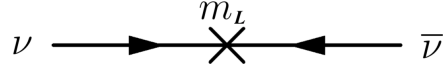
Figure 2.5: Feynman diagram showing the propagator -m_L \bar{\nu}_L^C \nu_L for the Majorana mass term [26]
