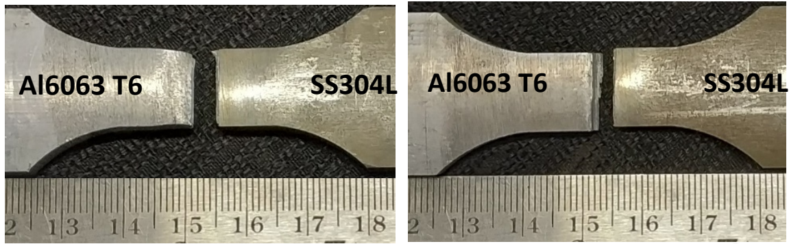
Figure 7. Fractured tensile specimens of sample 3
