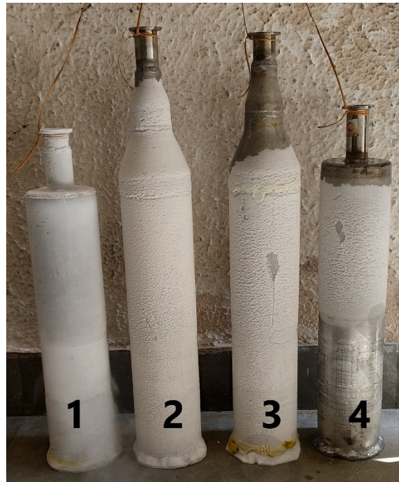
Figure 4. Samples after cryogenic thermal shocks
