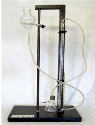
Fig. 2. Calcimeter instrument used to determine carbonate content.
