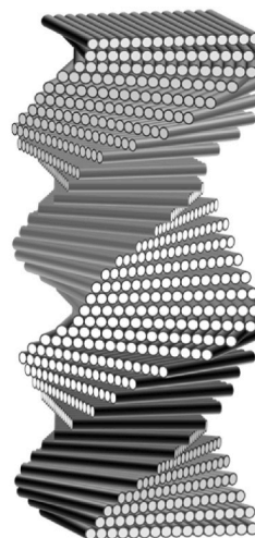
(b) Bio-inspired (BI) helicoidal design
