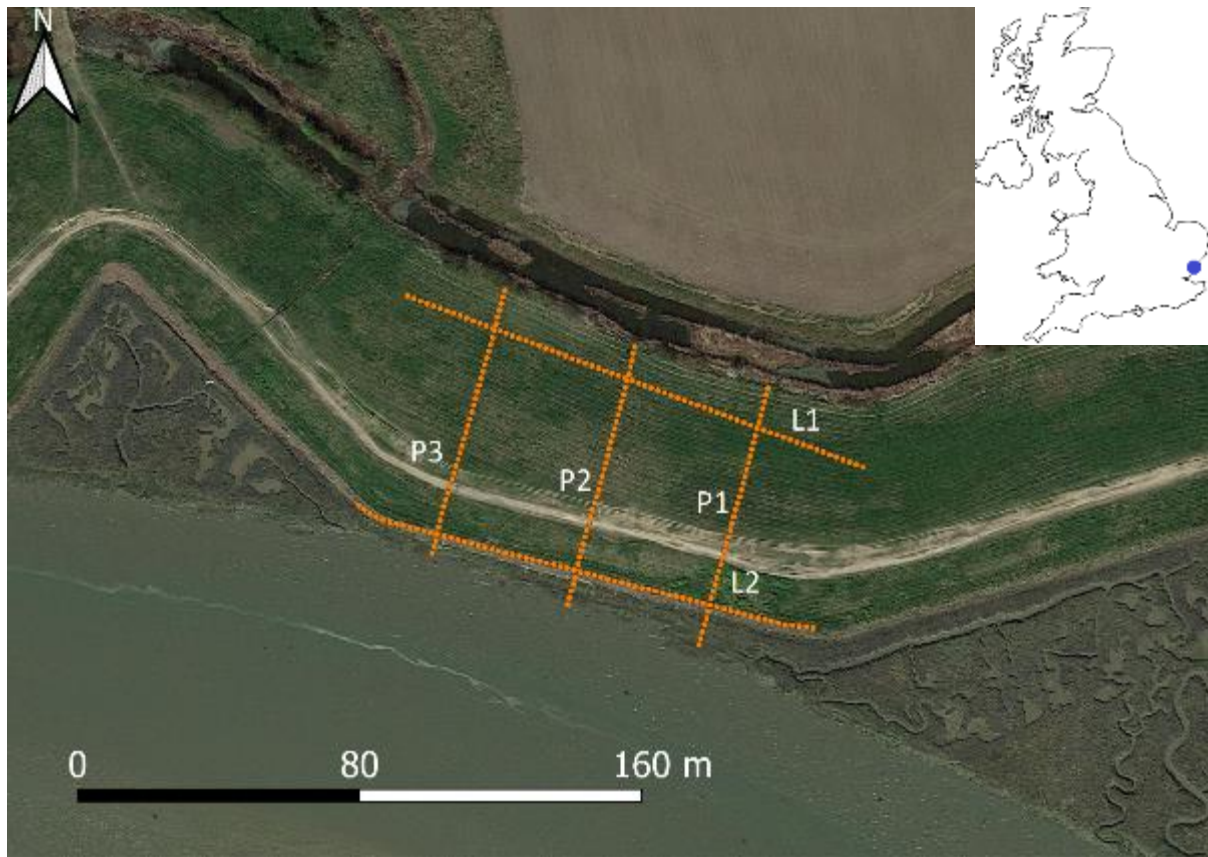
Figure 3.6: Layout of the PRIME array at Hadleigh Marsh, Essex, where L1-L2 are ERT lines parallel to the river front and P1-P3 are ERT lines perpendicular.
