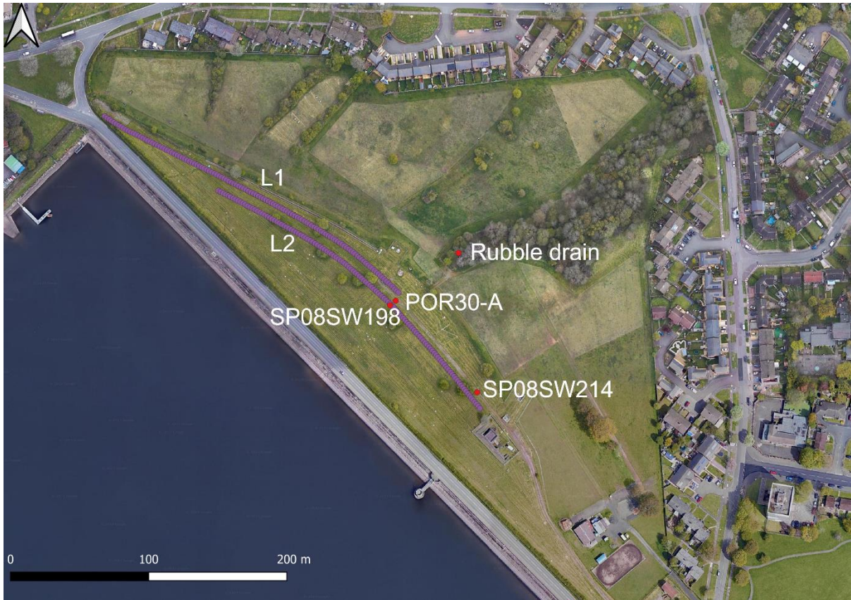
Figure 5.4: Location of the two major electrode lines, Line 1 and Line 2, at Bartley Dam. The map also shows a rubble drain, a piezometer (POR30-A) and two boreholes (SP08SW194 and 214) used for acquiring water flow rates, water levels and geological information.
