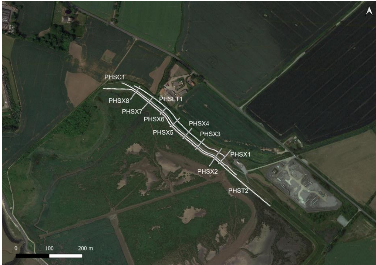
Figure 6.3: Electrode lines used for the ERT survey at Paull Holme Strays, where PHSLT lines are those parallel to the crest and PHSX lines are crosslines perpendicular to the embankment.
