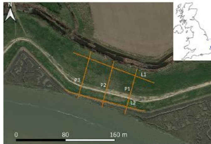
FIGURE 6 Layout of the PRIME array at Hadleigh Marsh, where L1 and L2 are ERT lines parallel to the riverfront and P1–P3 are ERT lines perpendicular.
