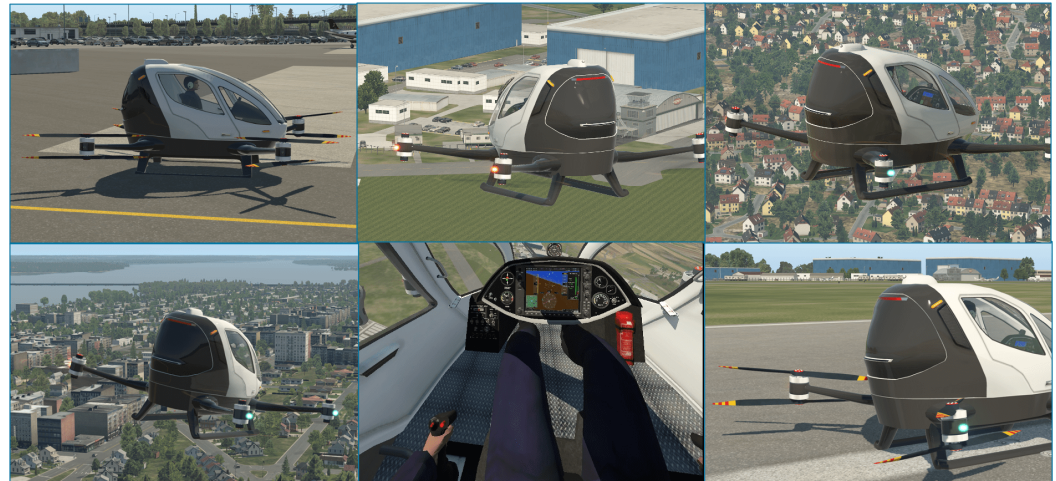
Figure 9. Vehicle simulated by the AAM simulator and passenger point of view from the VR headset.
