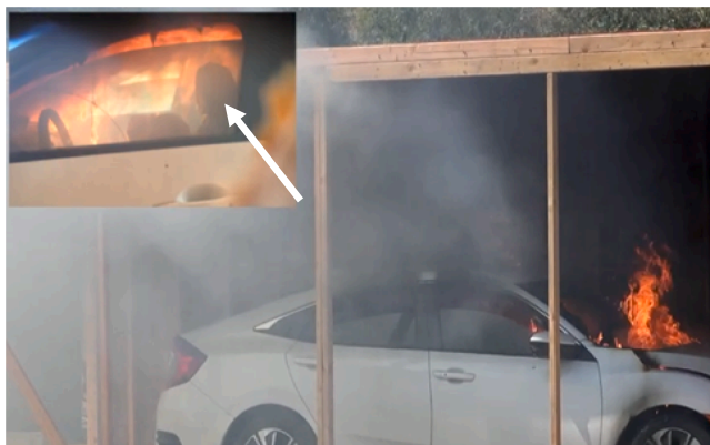
Fig. 12. Head in roof flame (indicated by arrow).
