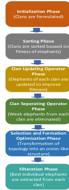
FIGURE 5. Block diagram - unfolding EHRE algorithm over scale-free IoT networks.
