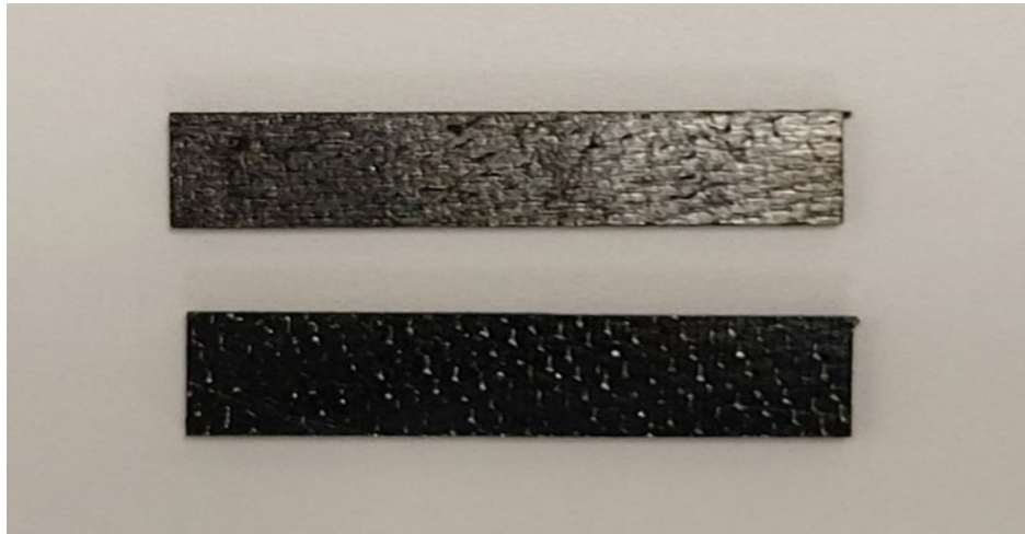
Figure 3-8 DMA coupon sizes cut from the manufactured sample.
