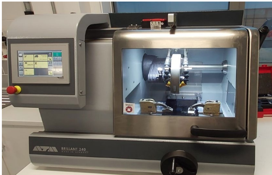
Figure 3-23 Glass/PFA sample cut using Brilliant QCUT 240A machine.
