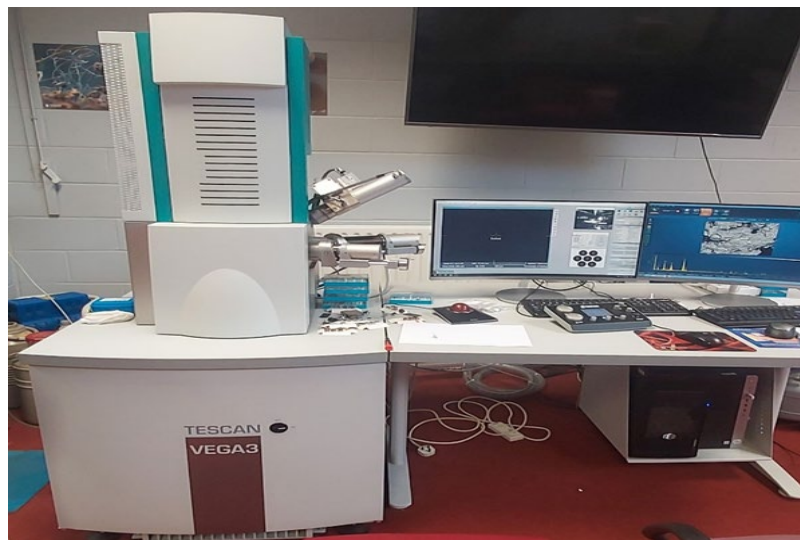
Figure 3-32 VEGA TESCAN 3 Scanning Electron Microscopy
