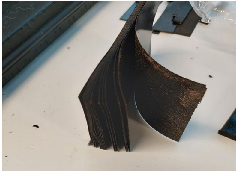
Figure 3-20 Glass/PFA sample manufactured via compression moulding without venting.
