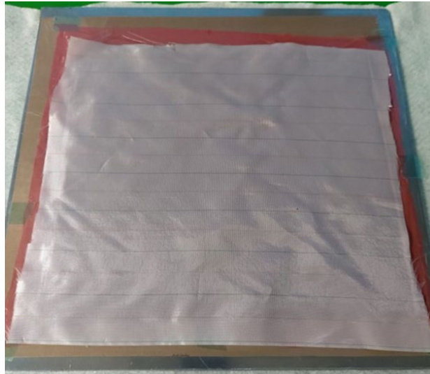
Figure 3-14 Layup setup covered with PA66 (Nylon 66) peel ply.
