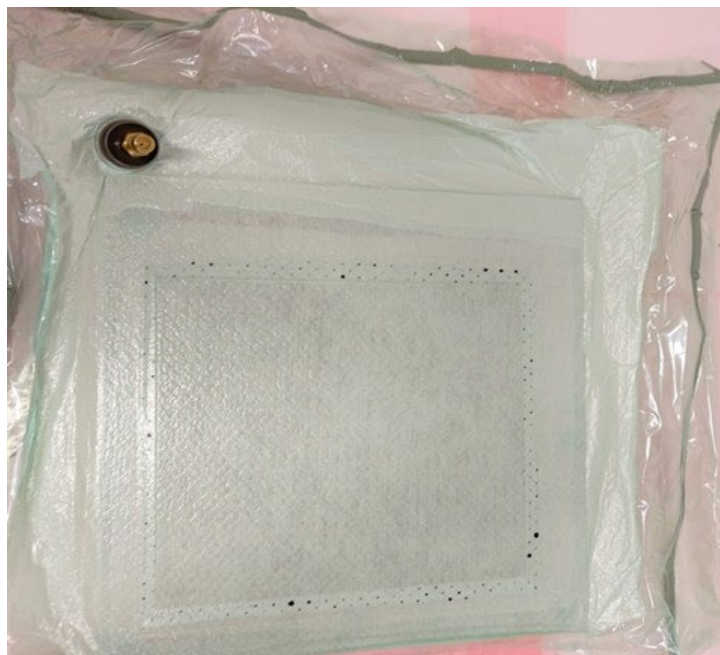
Figure 3-15 Vacuum bagged glass/PFA setup.
