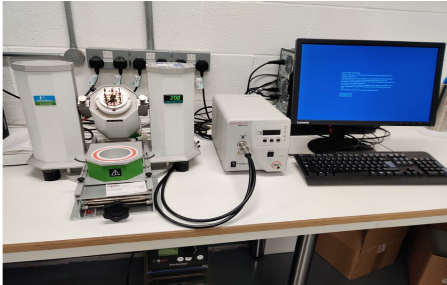
Figure 3-6. Perkin Elmer Dynamic Mechanical Analyzer (DMA) 8000
