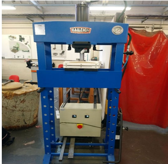
Figure 3-19 Lab-scale hot press
