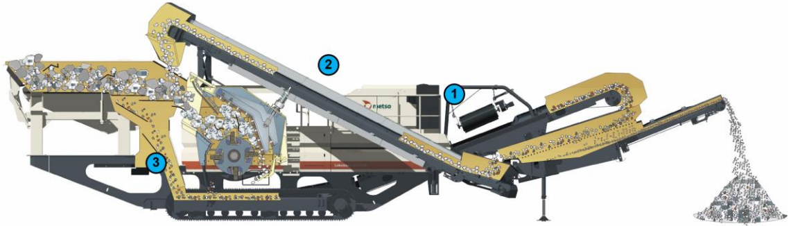
Figure 7. Microphone measurement locations (Modified from: Viilo, 2011)
