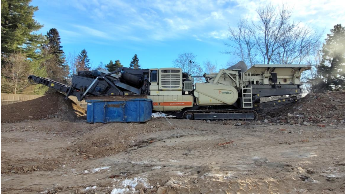
Figure 9. The mobile crushing plant used in the measurements. The feeder is located on the right and material flows from right to left.
