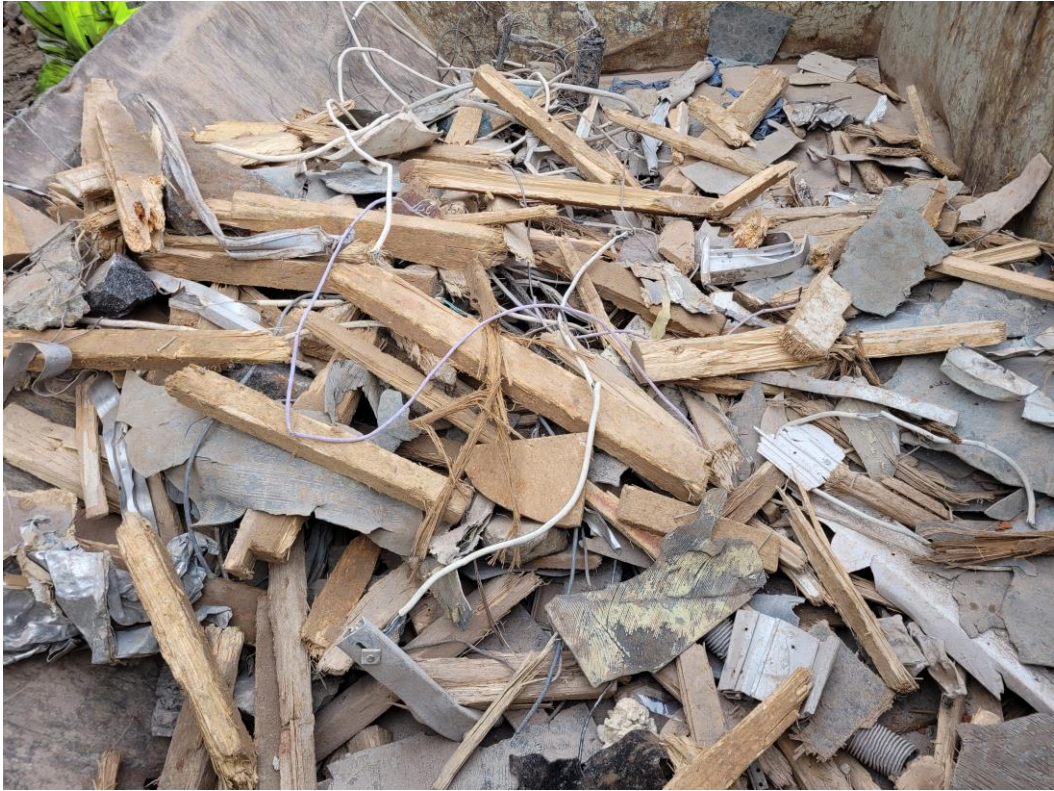
Figure 13. Light fraction by-product stream from the windshifter
