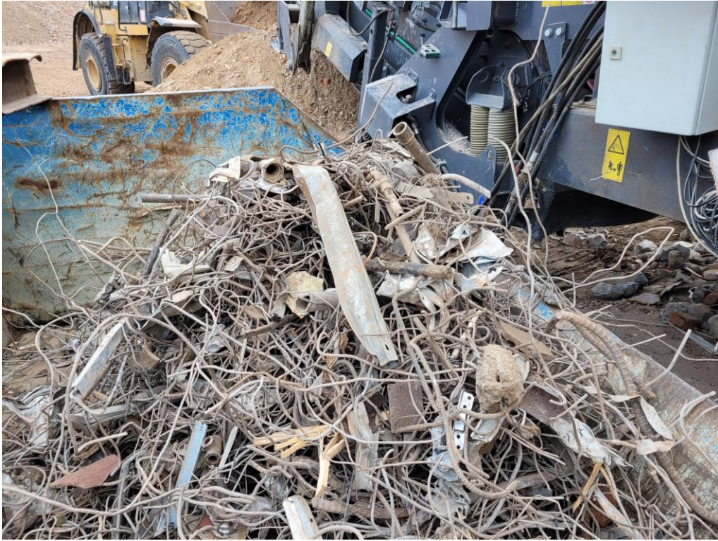
Figure 12. Metallic by-product stream separated by the magnetic separator.
