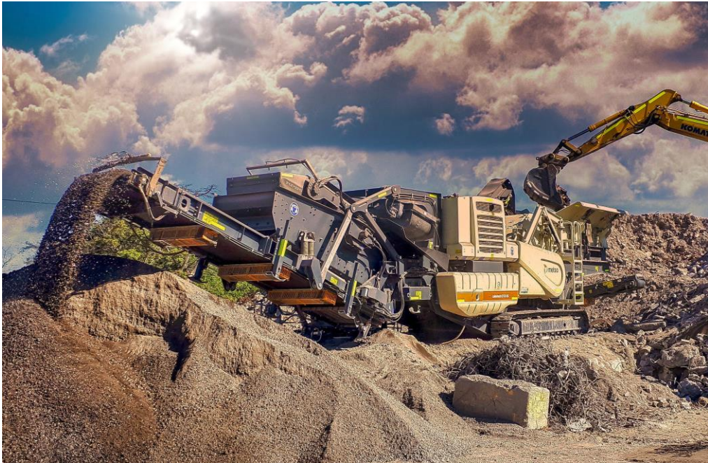
Figure 1. A mobile horizontal impactor crushing plant with a screen (Metso Outotec, 2022c)
