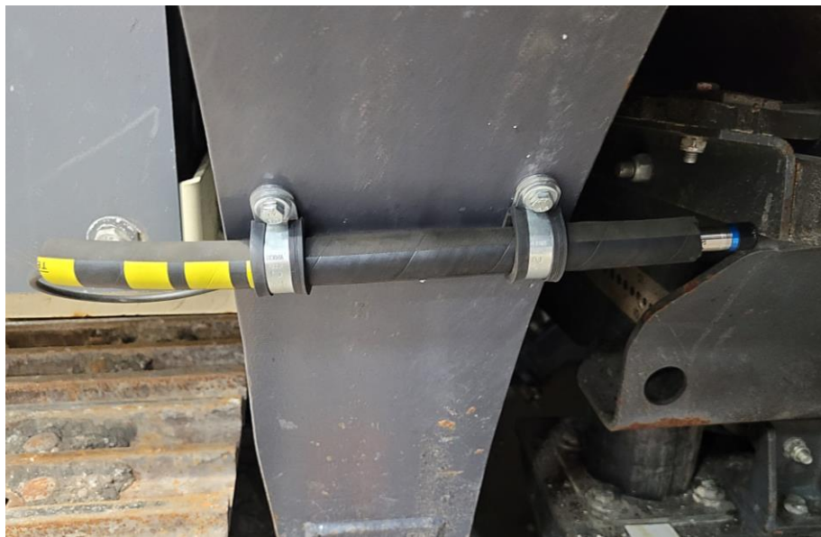
Figure 18. Mounting of the vibrating feeder microphone without windscreen.
