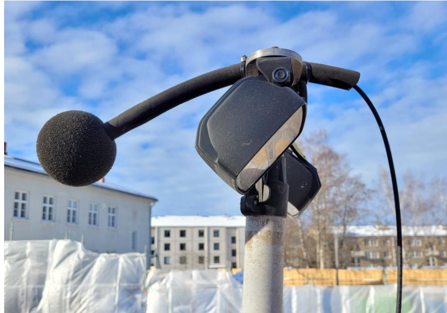
Figure 19. Mounting of the light mast microphone with windscreen attached.
