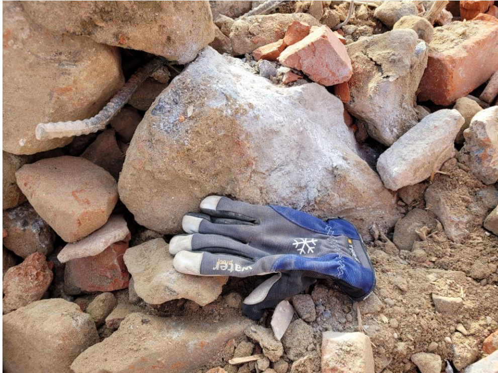
Figure 11. Feed material included different rocks, concrete, bricks, and other materials.
