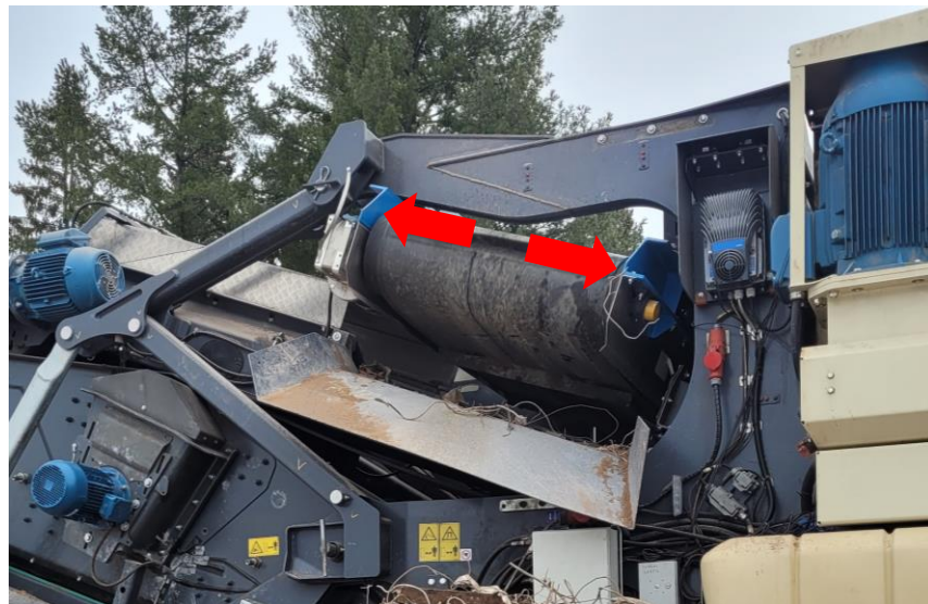
Figure 22. Magnetic separator. Rebar pieces were jammed between the frame (blue) and the belt and found their way along the entire circumference of the belt. Jammed rebar is not visible in this picture, and the gap between the frame and belt is illustrated with arrows.
