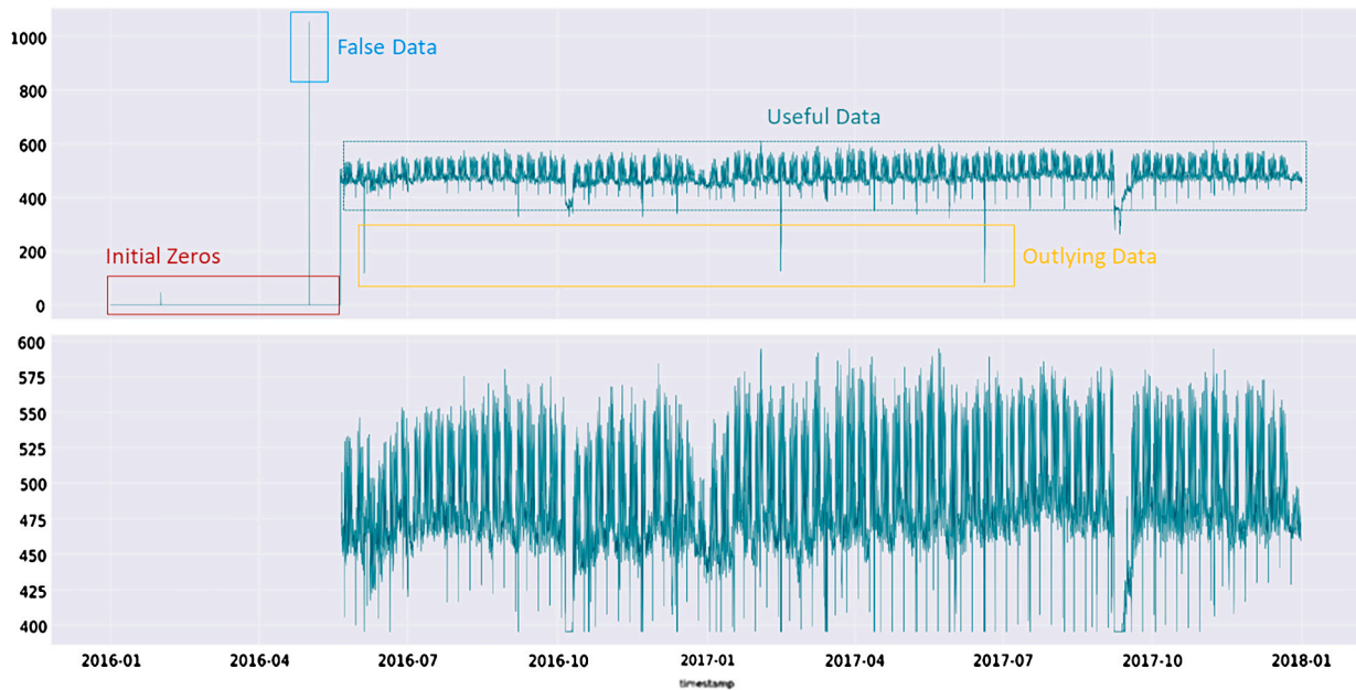
Fig. 4. Effect of Data Cleaning: Upper) Raw Data and Lower) Cleaned Data.
