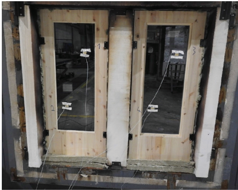
Figure 6. Photo showing positioning of thermocouples on the unexposed side of test specimens 04A and 04B.
