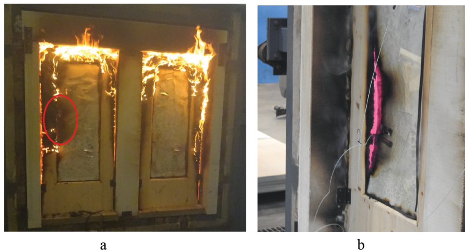
Figure 8. Close ups from the tests (a): 03A/03B after test termination. Cotton wool ignited in the marked area after 29.5 minutes, (b): 04A after 29 minutes, with sustained flaming and failure in temperature criteria.
