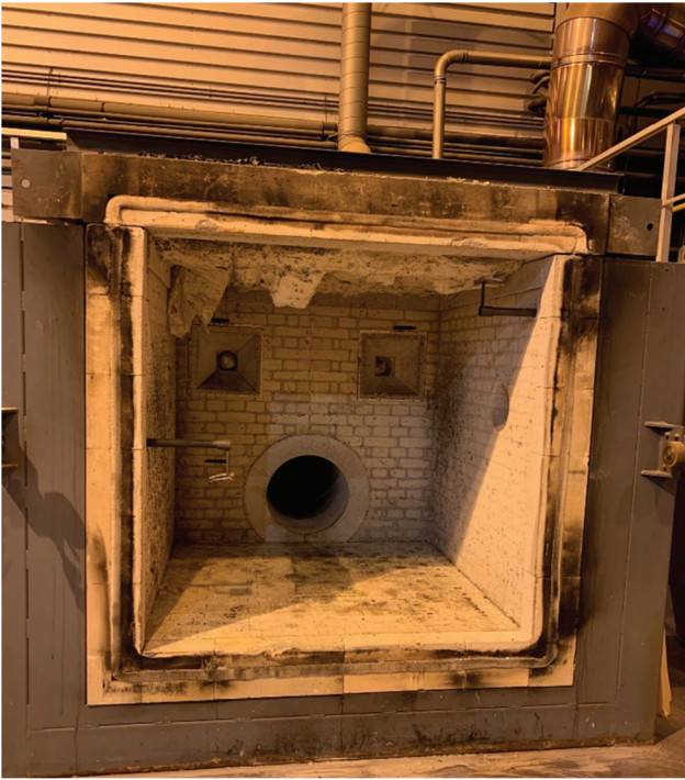
Figure 5. The fire resistance test furnace used for the tests.
