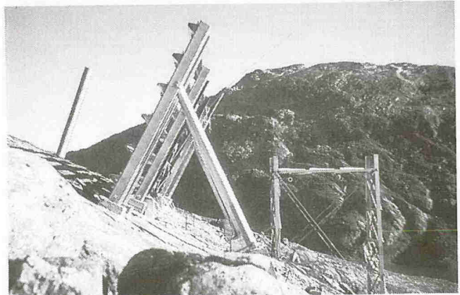
Fig. 6 Measurements of snow creep forces on steel structures
