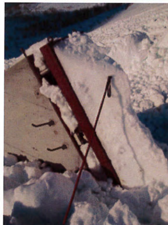
Figure 2.21: Avalanche 20050416 15:00: Sensor status before and after the event. Top: load cells at the steel tower; bottom at the concrete wedge. (Photos by Karstein Lied and Peter Gauer)
