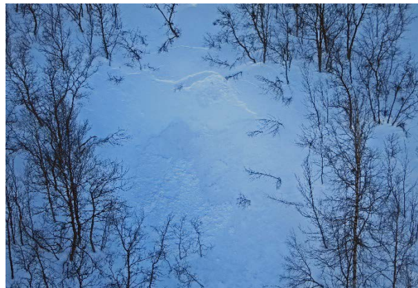
Fig. 1: Example of a result of DaisyBell explosion in a pocket inside birch forest. Only very small, near surface avalanches were released.
