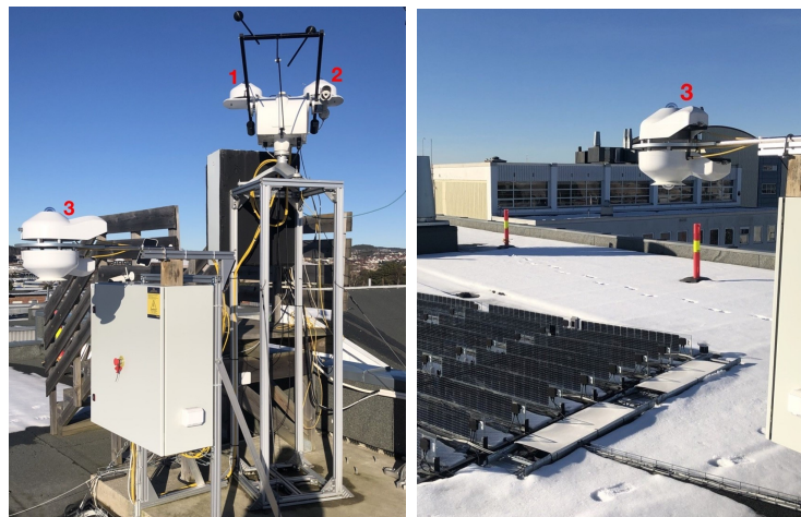
Figure 39: The pyranometer (1), pyr heliometer (2), and albedometer (3) relative to the test site.
