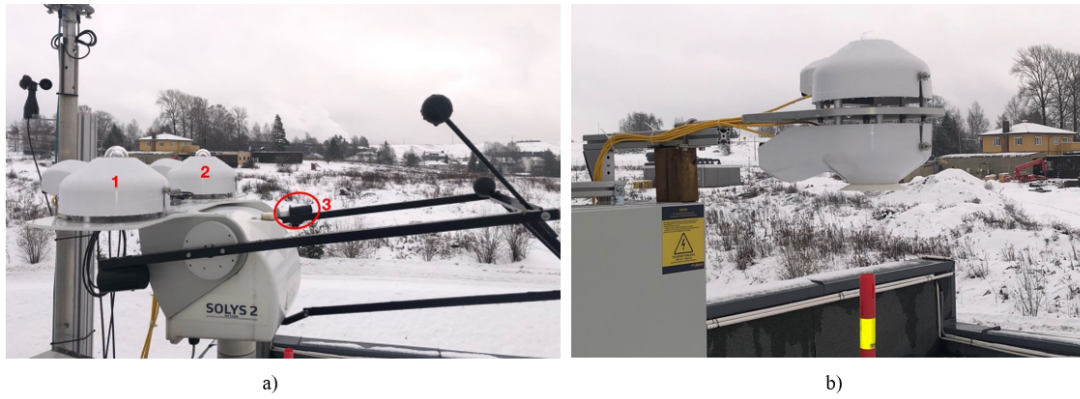
Figure 21: On picture a is the pyranometer (1) with an installed shading ball to measure DHI and the pyranometer (2) measuring GHI. The shading ball and the pyr heliometer (3) measuring the DNI are installed on a tracker. In picture b is the two pyranometers, for albedo, that measure the upwards and downward irradiance.
