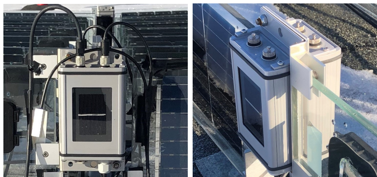
Figure 22: The reference cells at the test site from the front (left) and the side (right).
